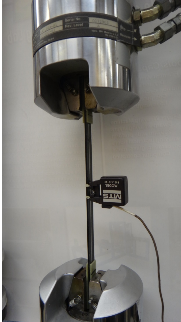
Figure 11. Composite Specimen During Testing
