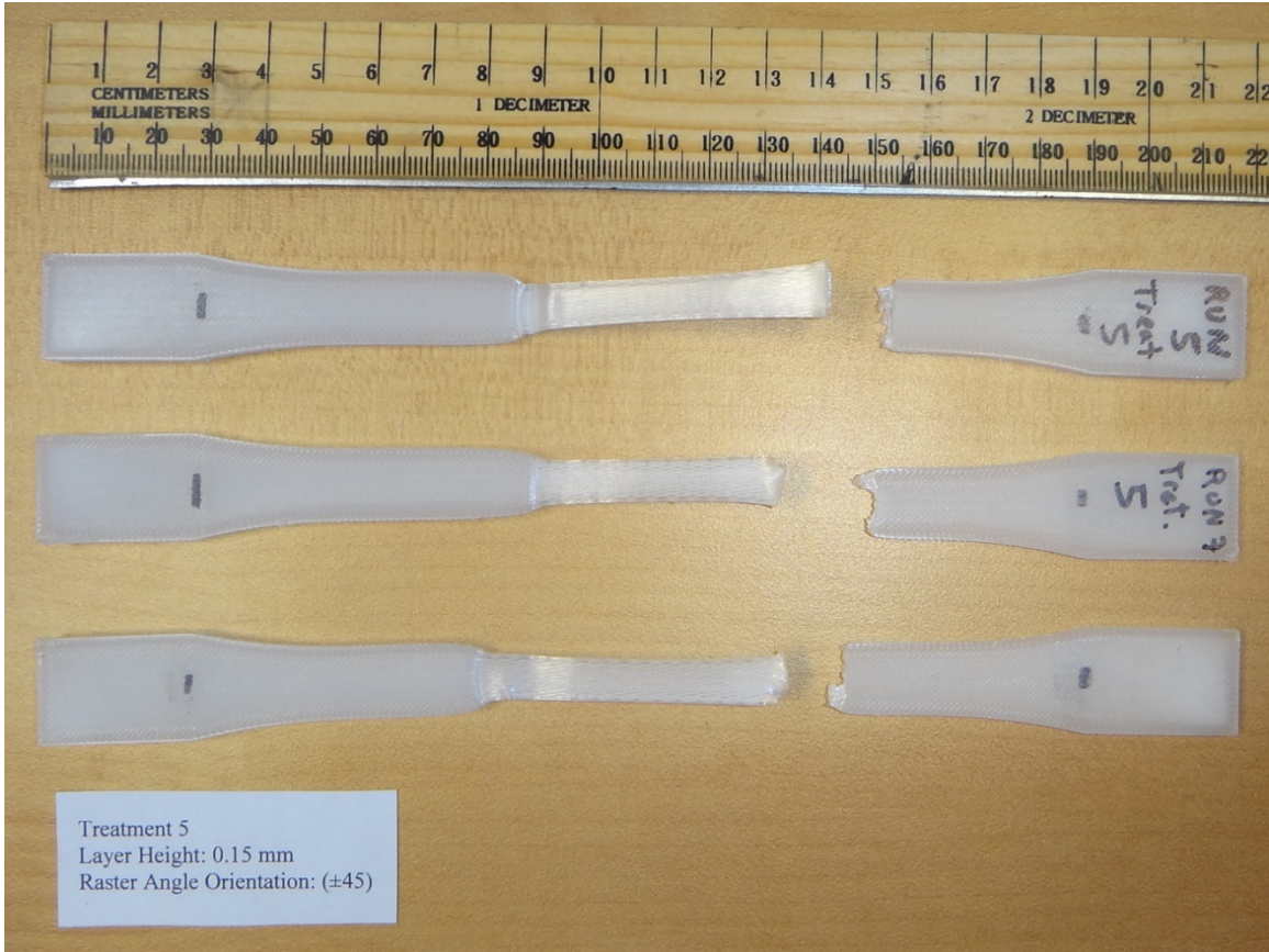
Figure 29. Treatment 5 Test Specimens after Testing
