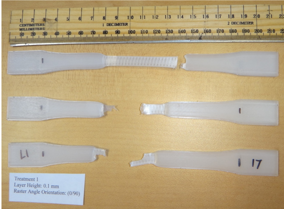
Figure 25. Treatment 1 Test Specimens after Testing
