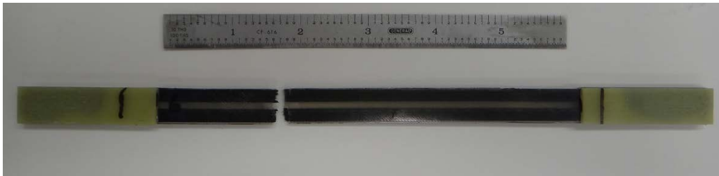
Figure 20. Continuous Carbon Fiber Composite Specimen After Testing
