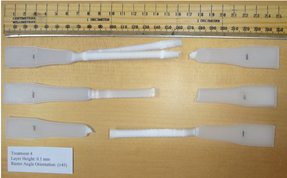
Figure 28. Treatment 4 Test Specimens after Testing
