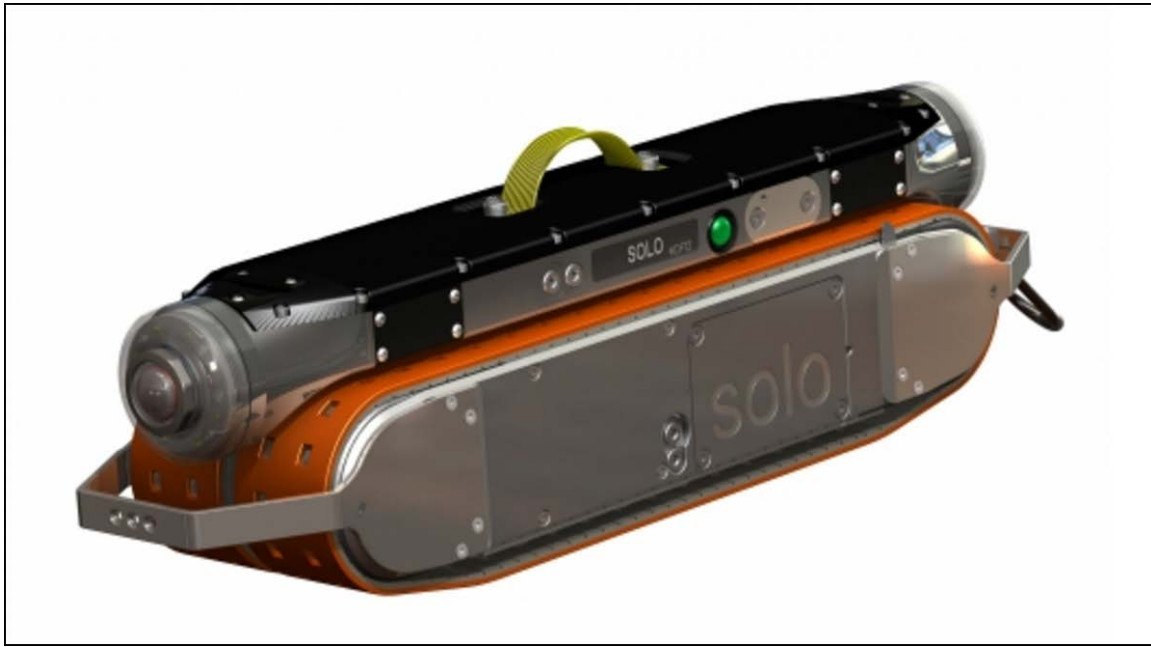
Figure 34. RedZone Robotics® Solo™ robot (RedZone-Robotics, n.d.)
