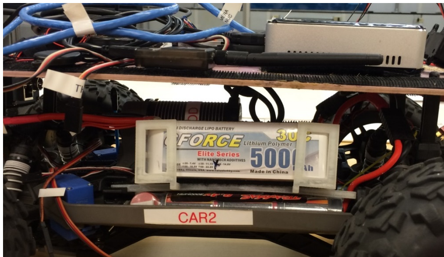
Figure 29. Autonomous Vehicle Battery Receptacle Attached to Robot
