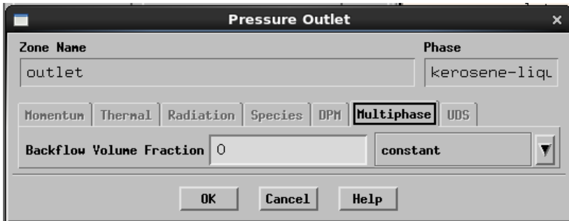
Figure 107. Fluent Settings: outlet multiphase settings (kerosene-liquid phase)
