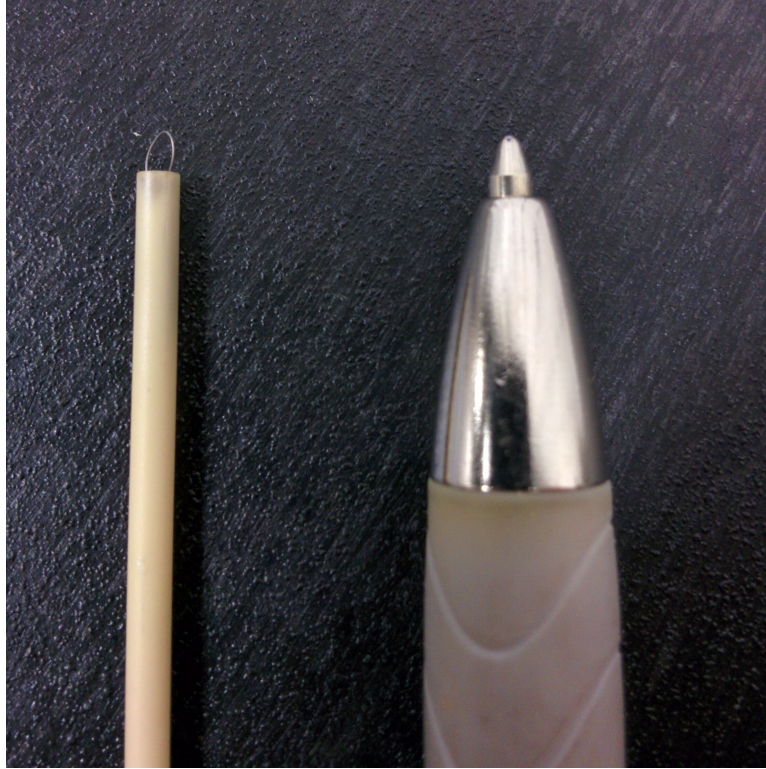
Figure 3.8: Emissive probe detail. Ballpoint pen for scale.
