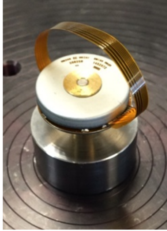
Figure 65. MOI Test Setup for Single Reaction Wheel and Motor
