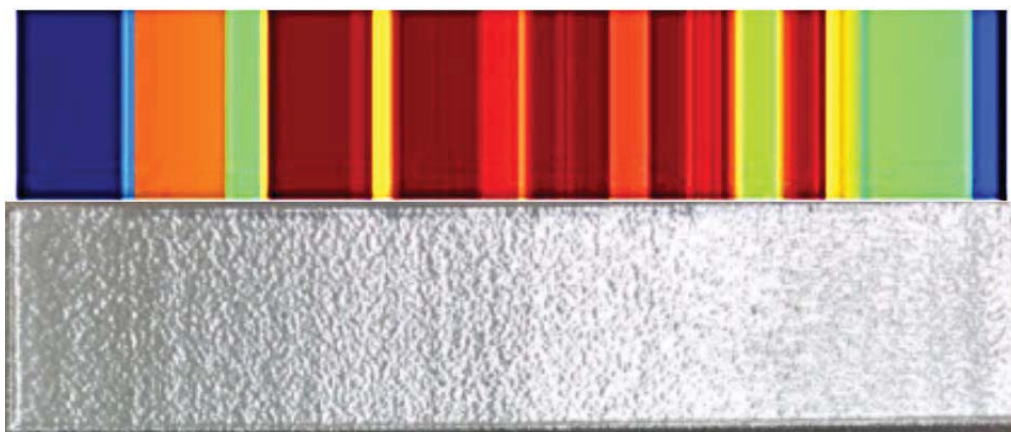
Figure 37. Beam current map compared to surface striations, Sample A-42 [39]
