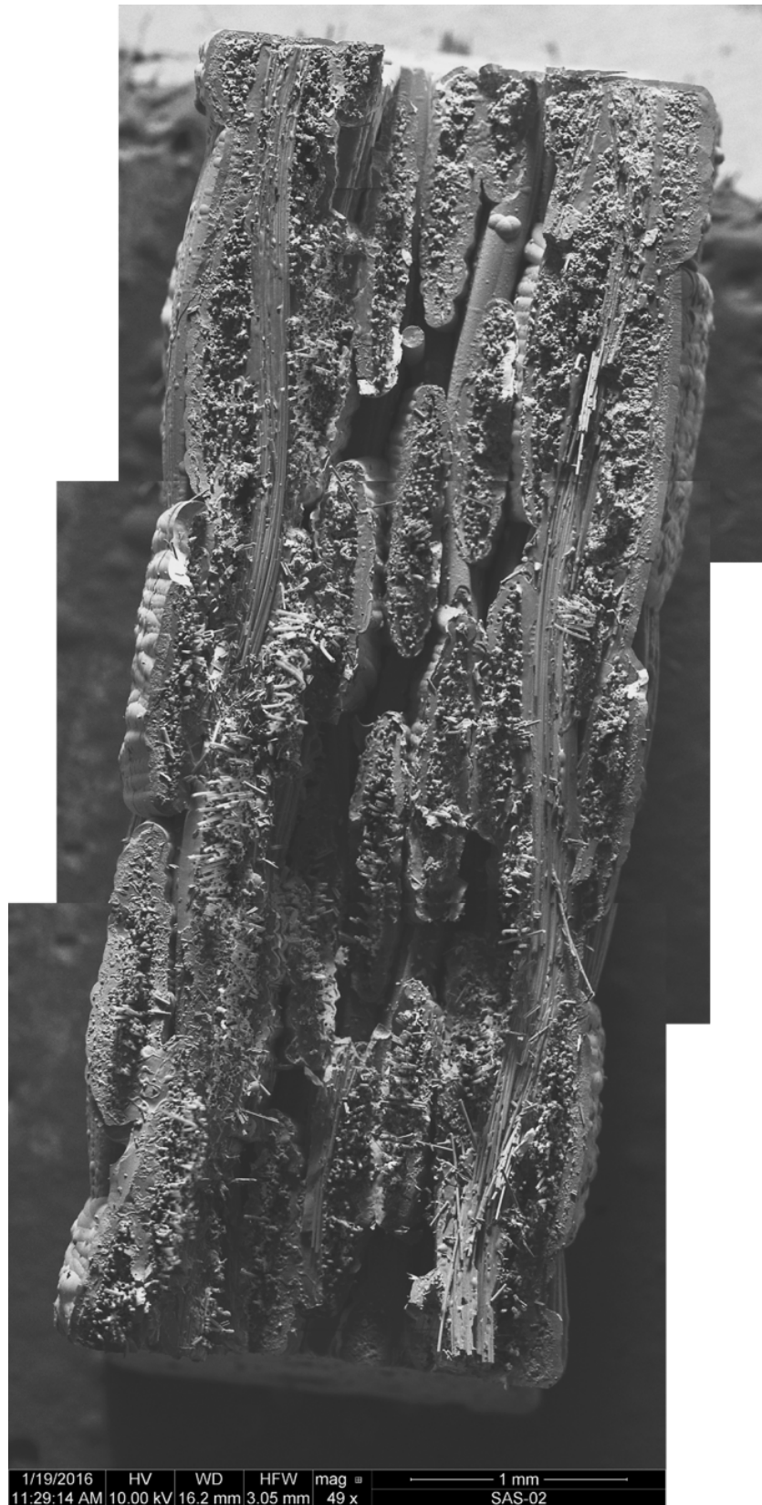
Figure 100: Fracture surface of the HG-shaped specimen tested in fatigue at 1300°C in air, \sigma_{\max} = 145 MPa, N_f = 68,831 , t_f = 19.1 h.
