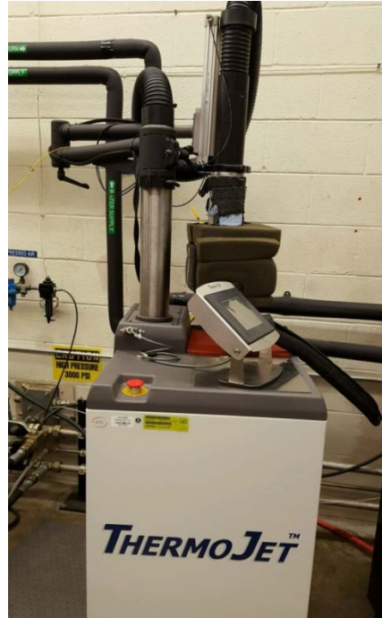
Figure 26. FTS ThermoJet ES for precision temperature cycles
