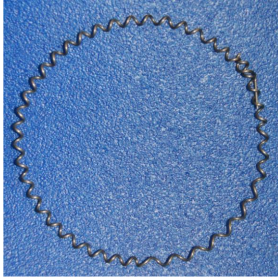
Figure A6.3 Photograph of the spiral inserted into the base of the detonation channel at the two o'clock position in the photograph and references to a 'spiral angle' indicate the location of this junction in the channel.
