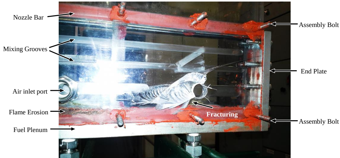
Figure A1.11 Flame erosion and sidewall fracturing of the polycarbonate mixing plenum sidewall at the sealed joint with the fuel plenum, following test H
