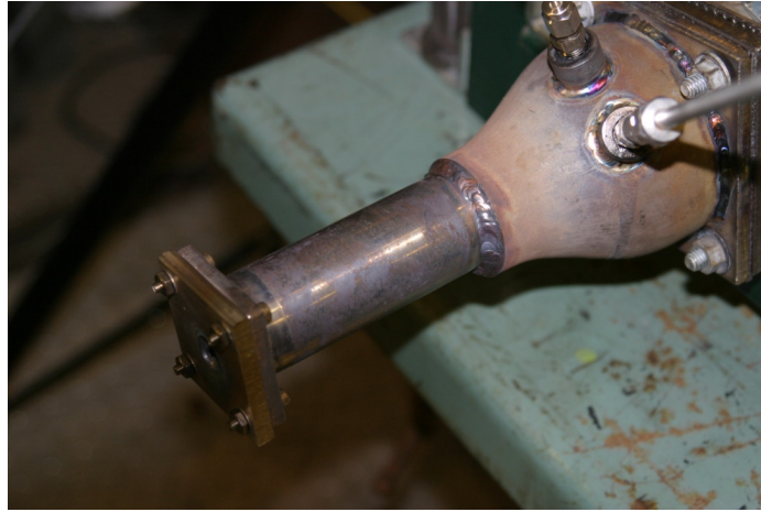
Figure 64. External Coloring on Reducer
