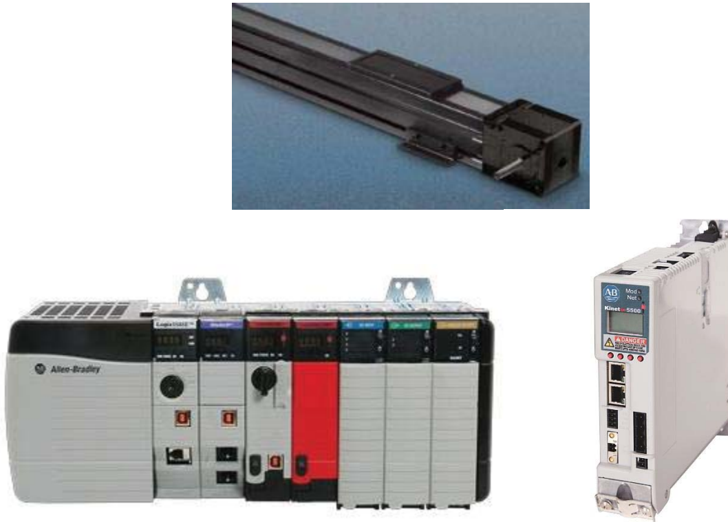
Figure 27. Experimental hardware. Top: Tolomatic belt-driven actuator. Left: Controllogix chassis setup. Right: Kinetix 5500 drive.
