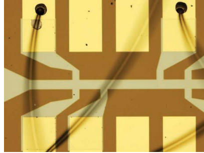
Figure 9: Optical microscope picture of the Hall bar. The gold rectangles are contact pads and the grey area is the channel processed using photolithograph. Leads are blurred due to optical diffraction.
