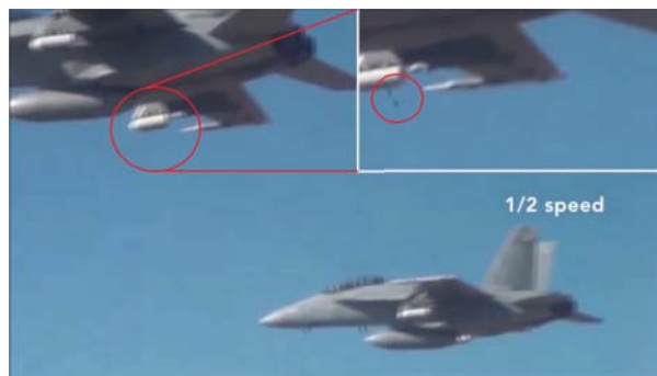
Figure 3: Recent DoD swarm demonstration [11] where small UAVs are launched from the small white pod attached under wing on a F/A-18 Hornet, these UAVs move so fast and are so small they are difficult to capture in an image.
