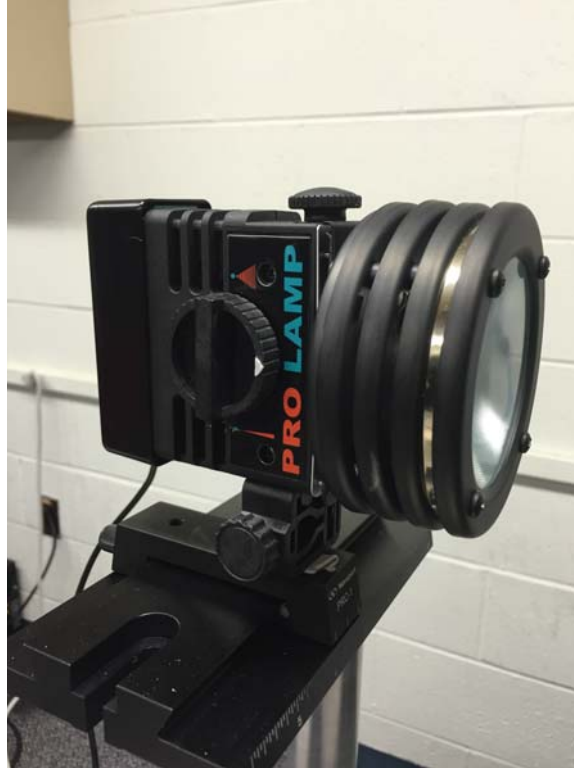
Figure 21. The ASD Pro Lamp is used as the light source in the image-based BRDF measurement system. The lamp has a 50 W quartz-tungsten-halogen bulb and is designed for indoor lab reflectance measurements over the region 350-2500nm.
