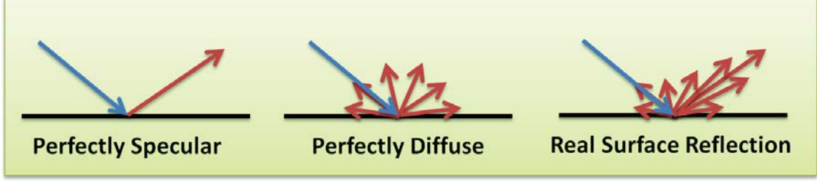
Figure 12. Three categories of reflectance: perfectly specular, perfectly diffuse, and the combination of diffuse and specular reflectance.
