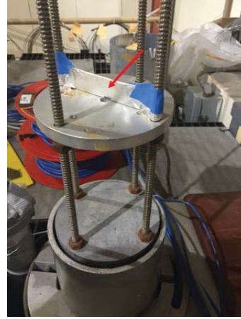
(b) Foil pack attached to rig for insertion into Co-60 source
