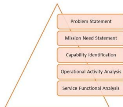
Figure 12. General DoDAF Architecture Development Process
