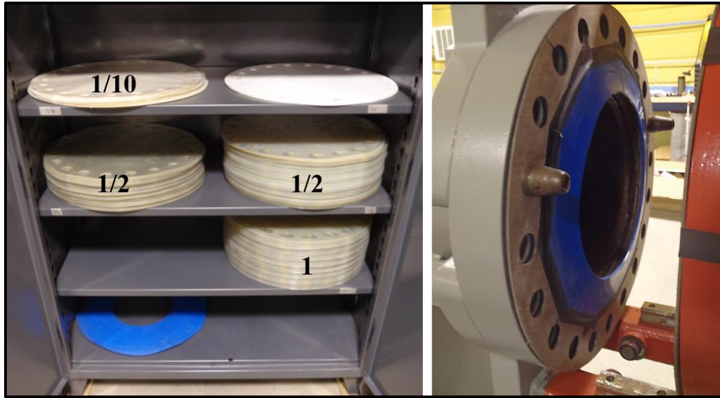
Figure 6. Mylar ® diaphragms (left) and the open breach in the shock tube (right).
