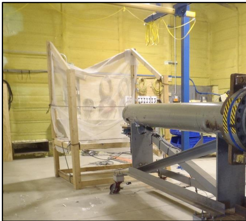
Figure 19. Catch net placed behind the test item position.
