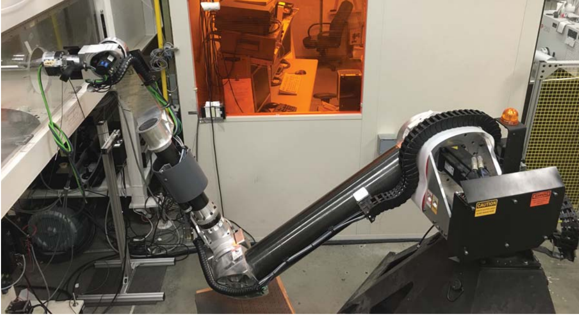
Figure 1. Motion Test Apparatus installed next to the AFIT Low-Speed Wind Tunnel
