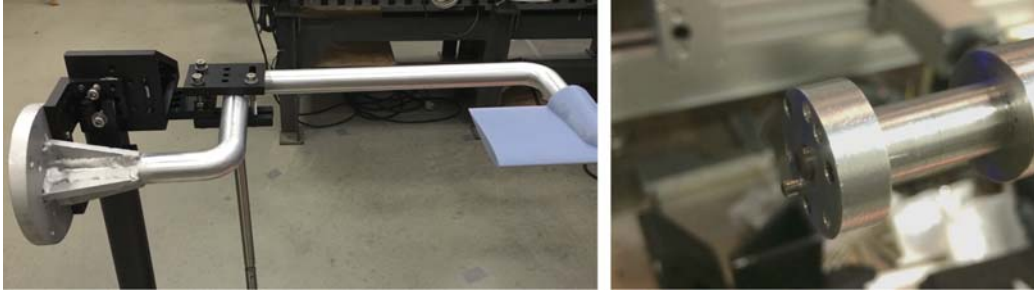
Figure 13. Model support sting with F/T transducer interface (right).
