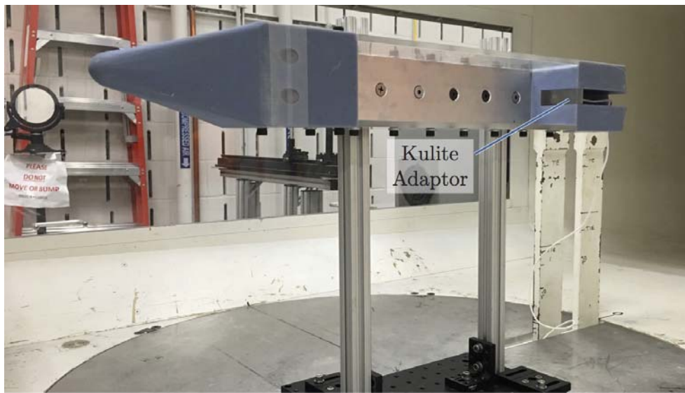
Figure 28. Installation of the small weapons bay for resonant frequency testing (shown with old Kulite transducer adaptor).
