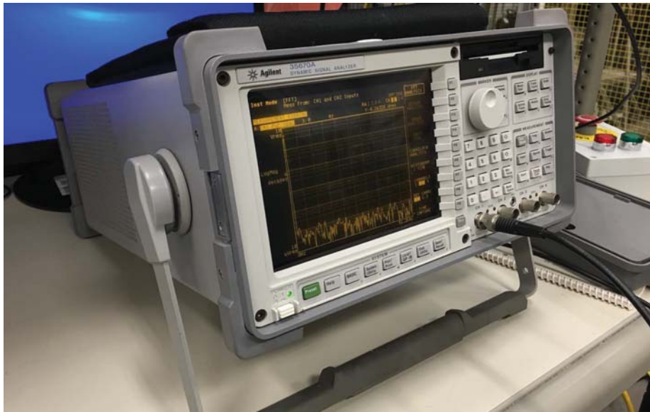
Figure 30. Agilent 35670A Dynamic Signal Analyzer used for resonant testing.
