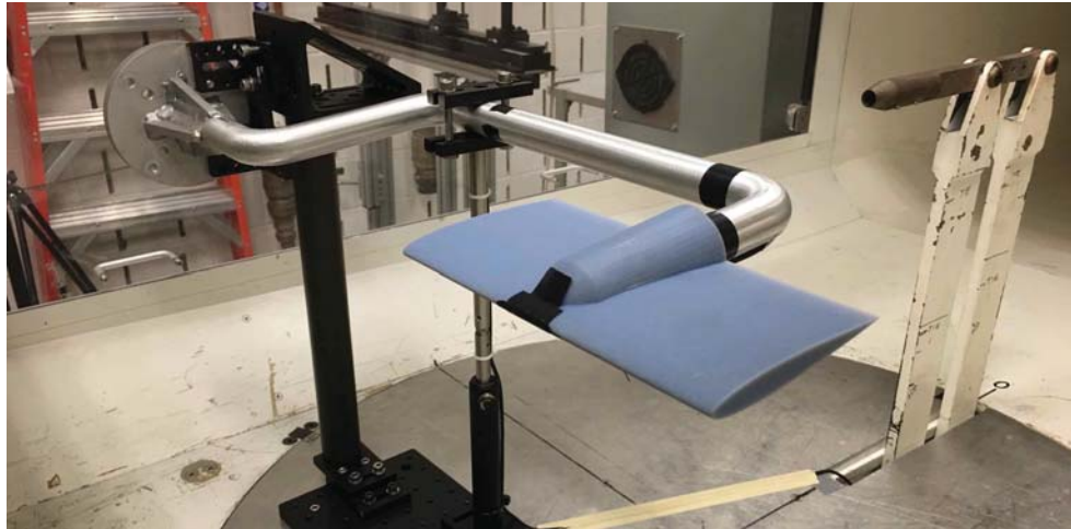
Figure 25. NACA 0012 Wind Tunnel test rig for taking measurements from the Nano25 at various angles of attack.
