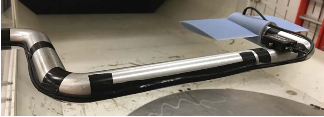
Figure 32. Detail of cable routing on back of sting.
