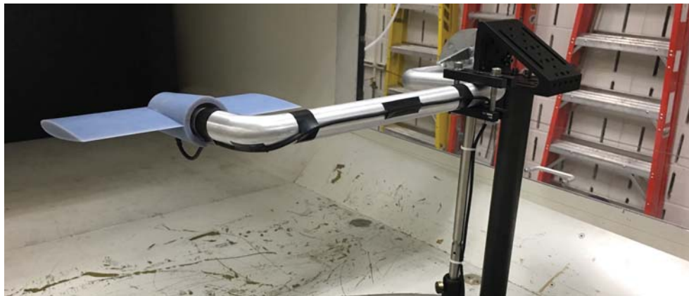
Figure 26. Rear of NACA 0012 wing model showing cable exit and path along sting.
