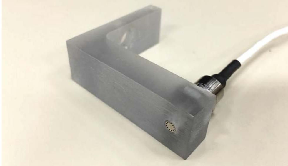
Figure 29. New adaptor for installing Kulite pressure transducer in rear surface of the small weapons bay.
