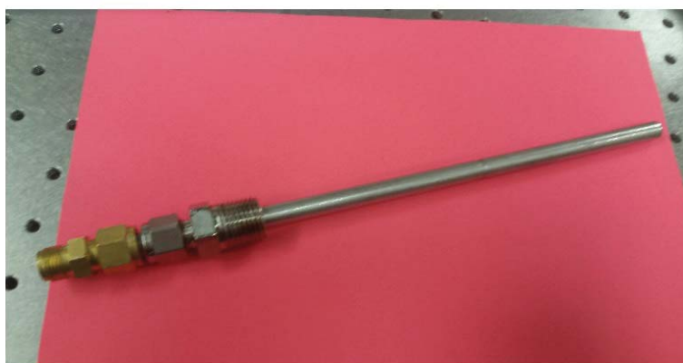
Figure 28. Shroud tube schematic (Top) and reference picture (Bottom)
