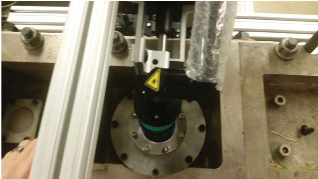
Figure 25. Laser light entry from the top of the wind tunnel test section
