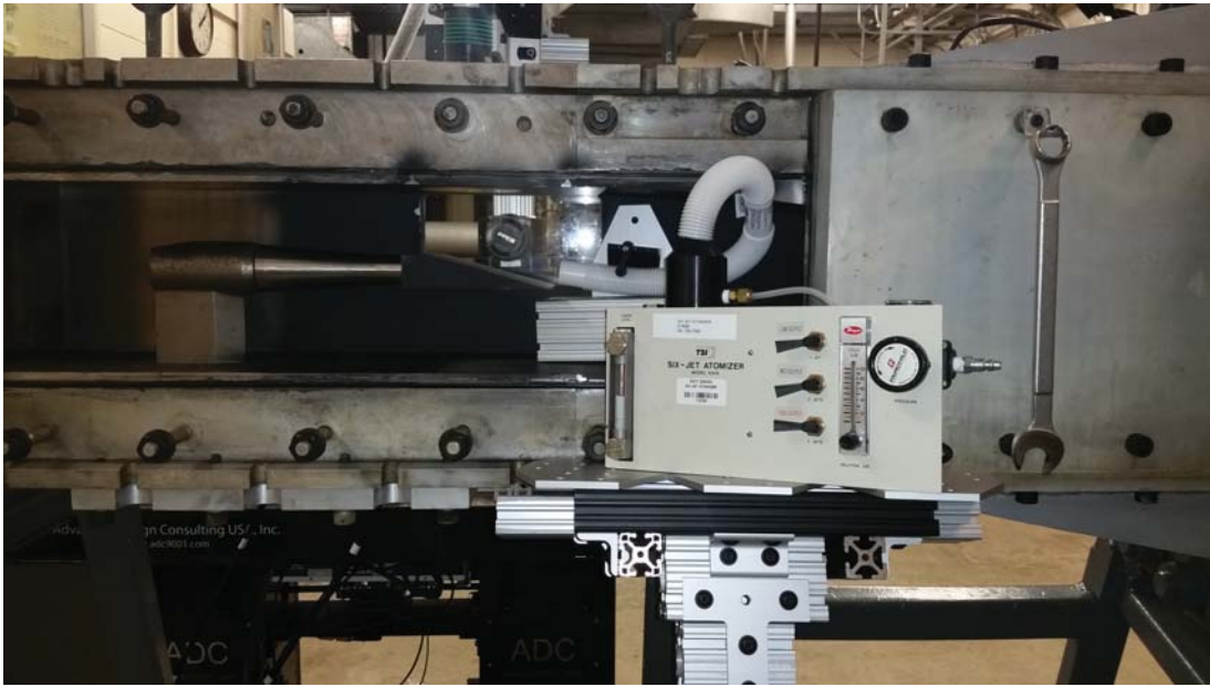
Figure 31. Calibration configuration with 6 jet atomizer in test section
