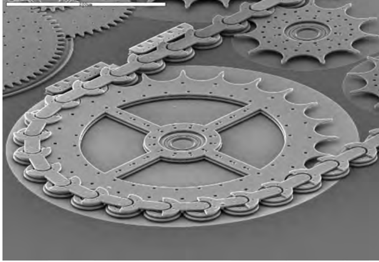
Figure 11. This is an sample device that can be made by the SUMMIT V fabrication process. The multilevel process allows four layers of polysilicon to be deposited, allowing the fabrication of rotors, joints, and gears. Numerous designs from multiple users can be fabricated in a single run, facilitating the supply of complex MEMS structures to individual users [65].
