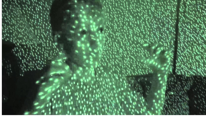
Figure 15. Illustration of Kinect's IR Dots by [8]
