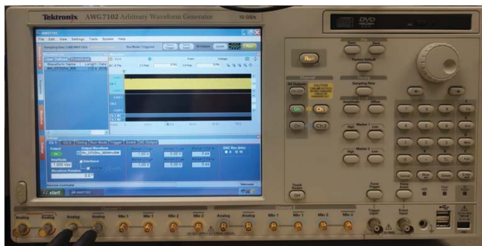
Figure 12. Tektronix Arbitrary Waveform Generator - AWG7102 used to generate the radar LFM waveform.
