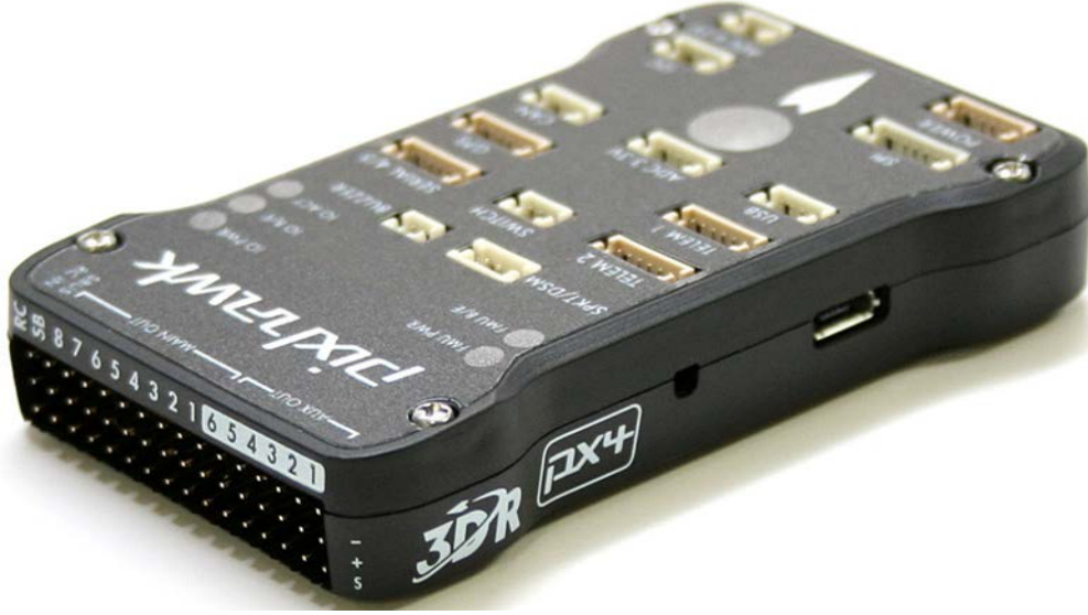
Figure 7. Pixhawk Autopilot Used for UAV Navigation [4]
