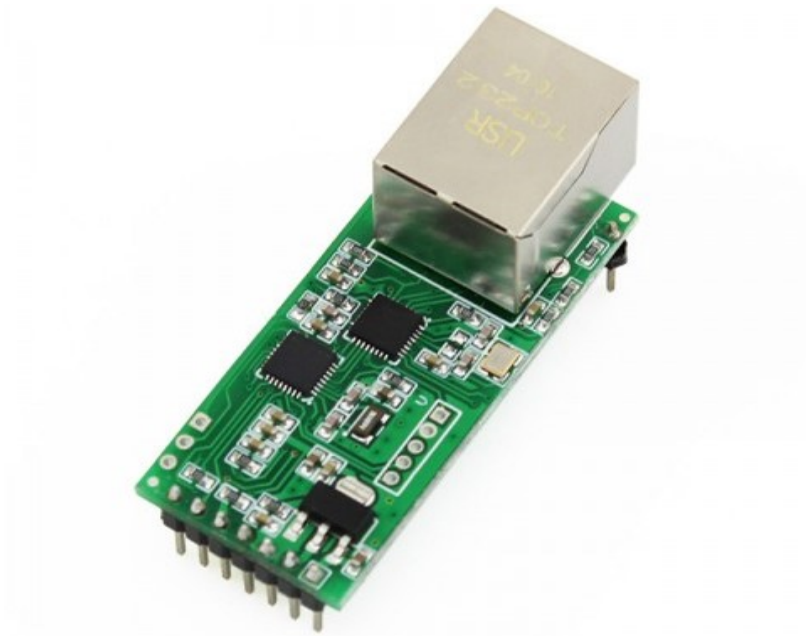
Figure 9. UART Serial Ethernet Module for the Pixhawk Data Collection [6]
