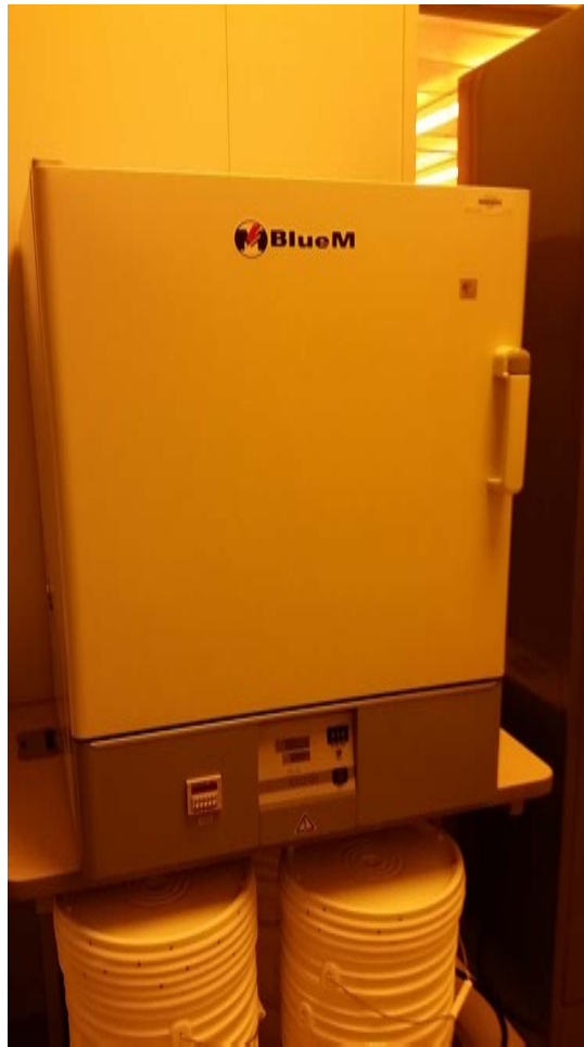
Figure C-8. Blue M standard convection oven for curing, moisture drying, and other processes and testing requirements
