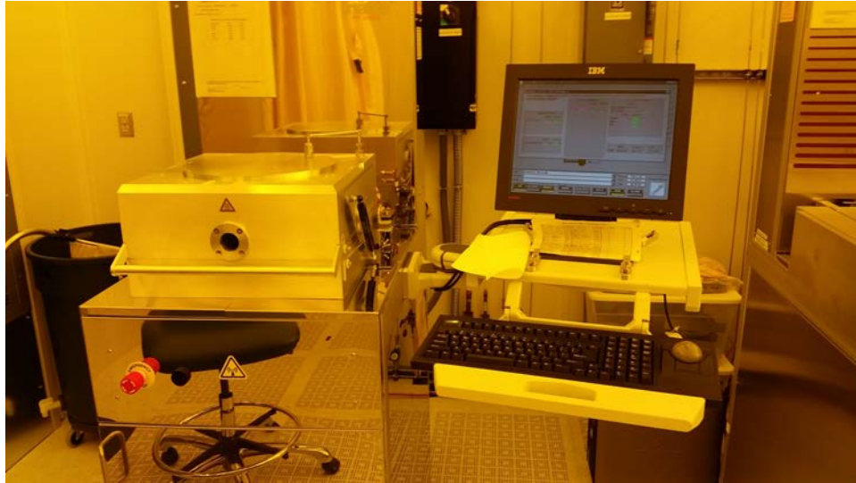
Figure C-5. The Unaxis 790 reactive ion etcher (RIE) is a general-purpose parallel plate plasma etching system which uses ionized fluorocarbon gases and oxygen to etch polymer and dielectric materials. It can also use argon to physically etch metals. The large chamber can accommodate substrates ranging from 200 mm diameter wafers down to small pieces
