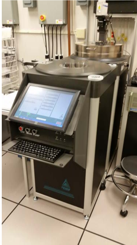
Figure C-4. The Minilock-Phantom RIE ICP is an advanced high density etching system with a vacuum loadlock and an inductively coupled plasma (ICP) source used for etching polymers and dielectric materials. The ICP allows for improved anisotropy in high aspect ratio structures
