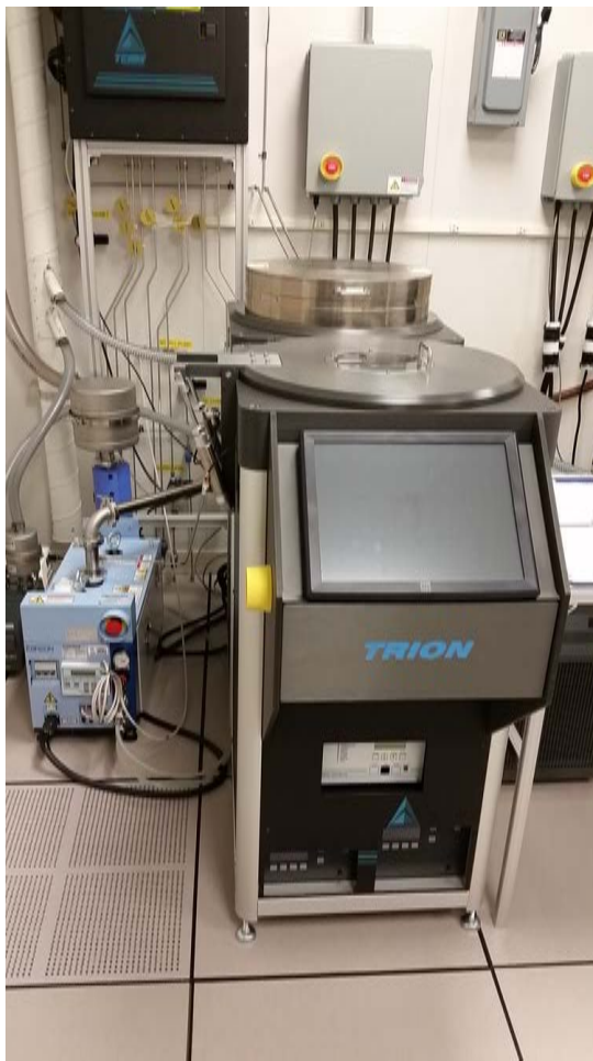
Figure C-6. Minilock-Orion is a plasma-enhanced chemical vapor deposition system. The heated vacuum loadlock stage of this system was utilized in order to anneal the P(VDF-TrFE) copolymer
