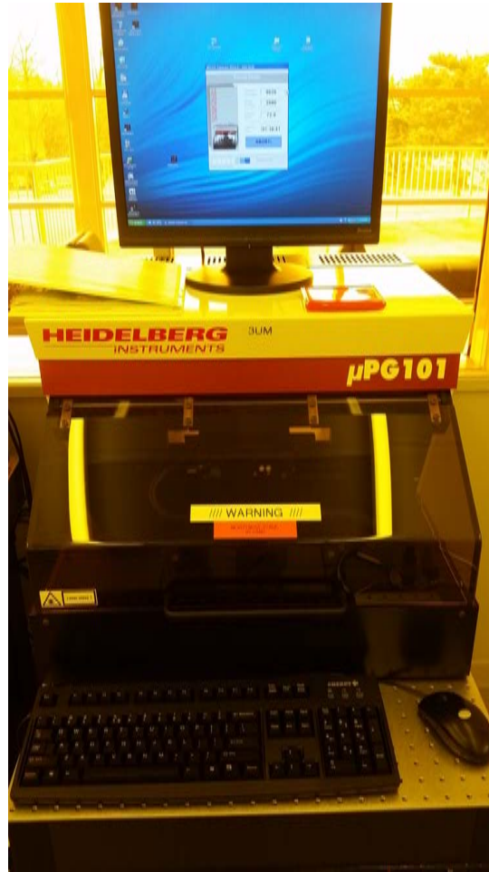
Figure C-1. Heidelberg \mu PG 101 Mask Writer used for printing 4" masks used in this research
