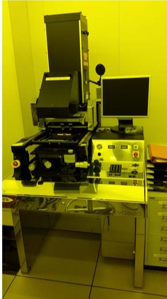
Figure C-3. The EVG®620 Automated Mask Alignment System is a tool designed for optical double-side lithography and precision alignment up to 150 mm wafer sizes.
