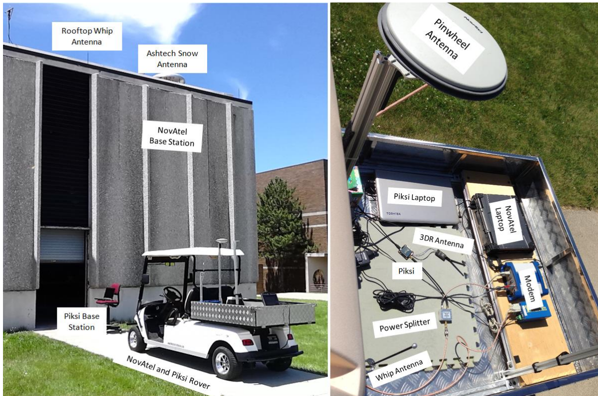
Figure 13. NovAtel and Piksi Characterization Apparatus
