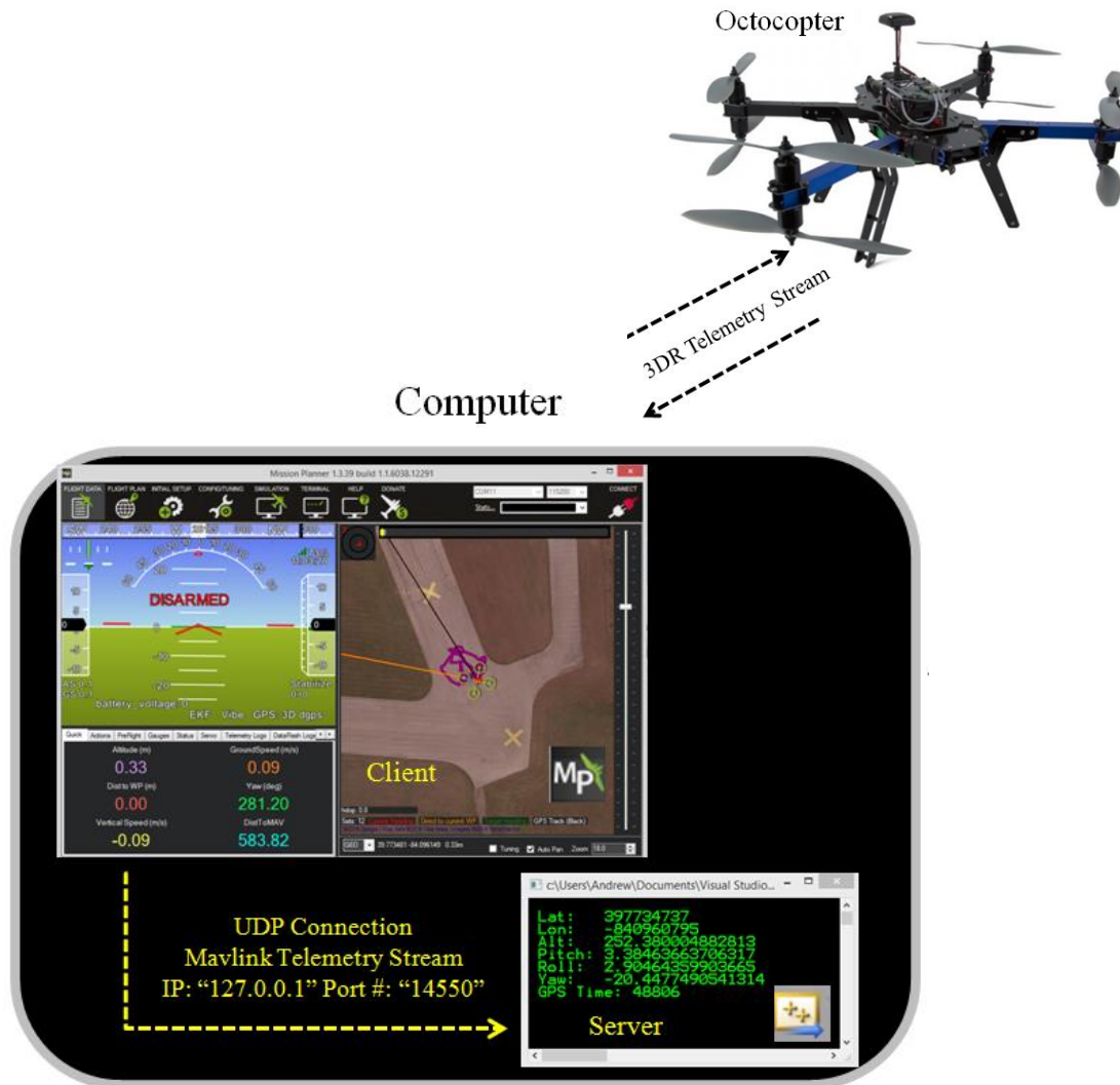
Figure 17. Position-Pose Alignment System Architecture
