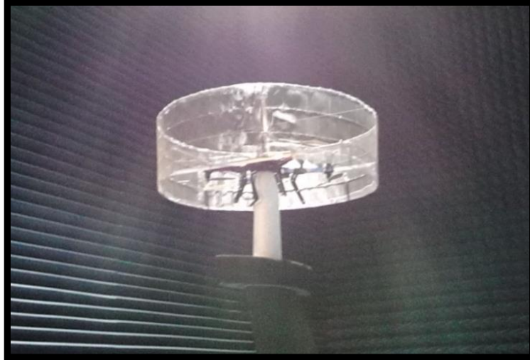
Figure 26. ACER Facility, Shielded Octocopter mounted on Cylinder Foam Column
