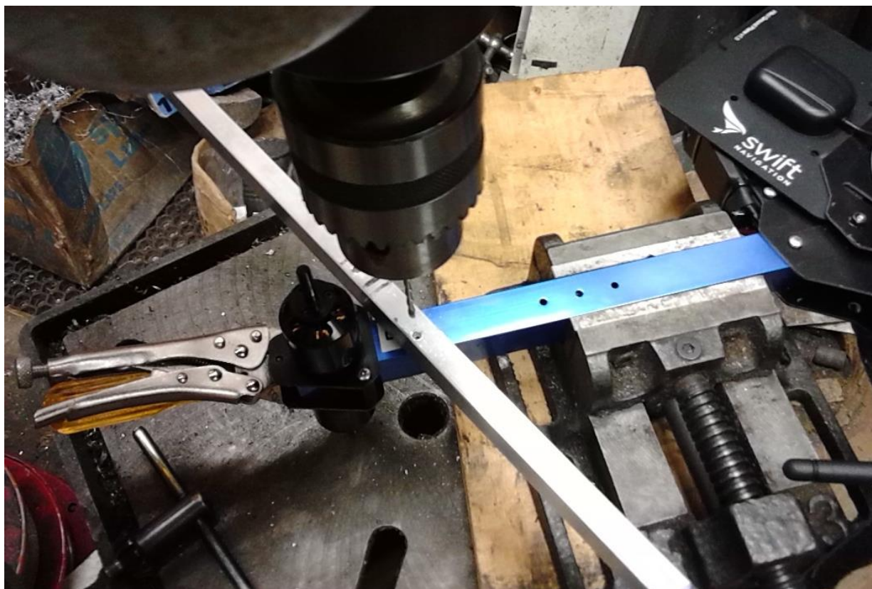
Figure 22. Modifying the X8 octocopter frame with L channel extensions
