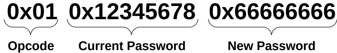
Figure 14. Reverse-engineered Safetech command structure at the HCI level.
