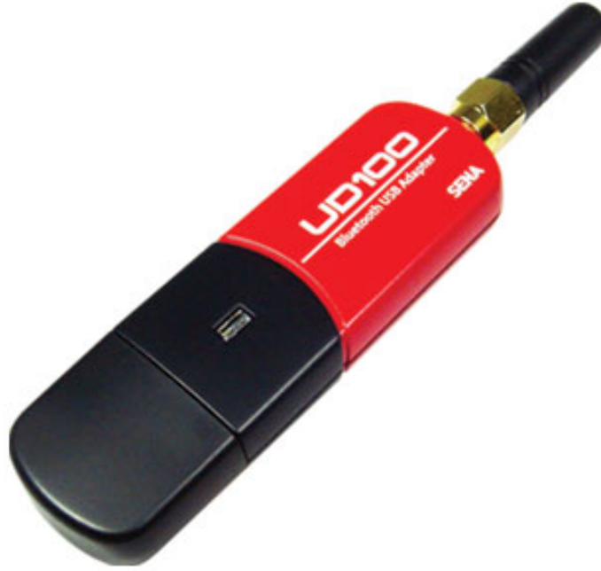
Figure 7. The Sena UD-100 Class 1 Bluetooth adapter with optional detachable antenna used for range-finding experiments and long-range Bluetooth communication.
