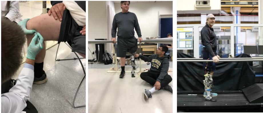
Fitting and alignments of device to patients. Biological knee joint center was measured on the intact side and the build height of the powered device was modified to allow for alignment of the rotation of the knee joint. Fittings and alignments have been performed on 4 individuals with transfemoral amputation to date.
