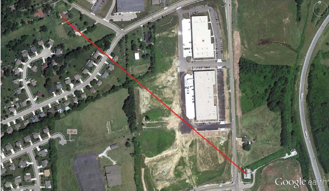
Figure 21. Satellite image of Transmitter to Receiver path for the first cell phone data collection location. The path length is 623m. The distance from the KILN radar (not shown) is 42km. Image copyright owned by ©Google 2015.
