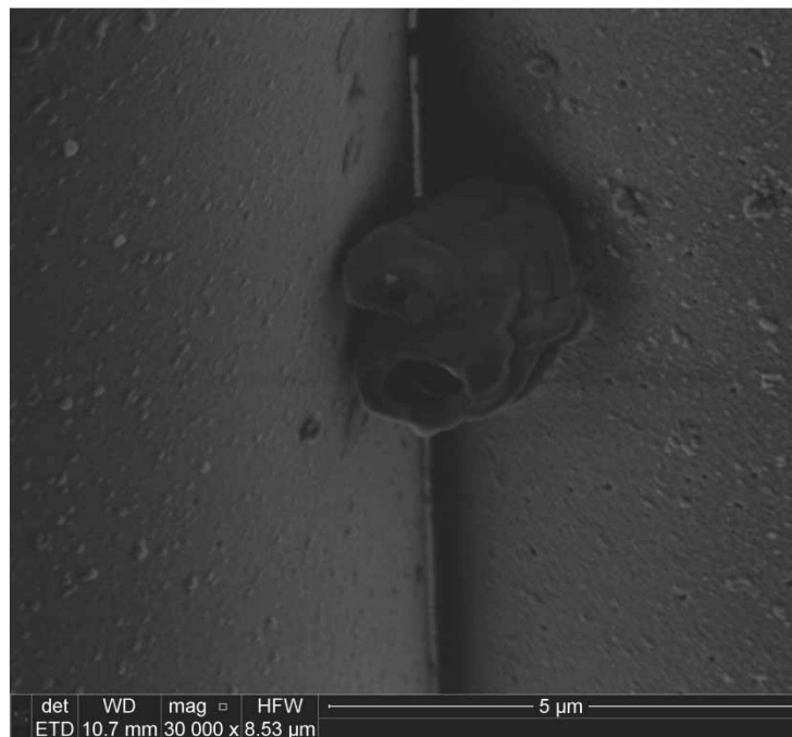
Figure 129. SEM micrograph of the Hi-Nicalon™ S specimen “Steam 4” examining a deposit that appears to be bound to two fibers, near the midpoint of the effective length. This deposit and these fibers are also shown in Figure 128
