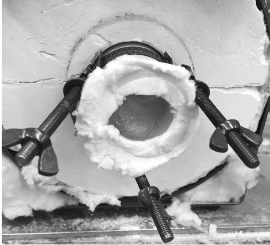
Figure 44. Cut, round piece of sheet insulation in place prior to attachment of steam generator to alumina tube.
