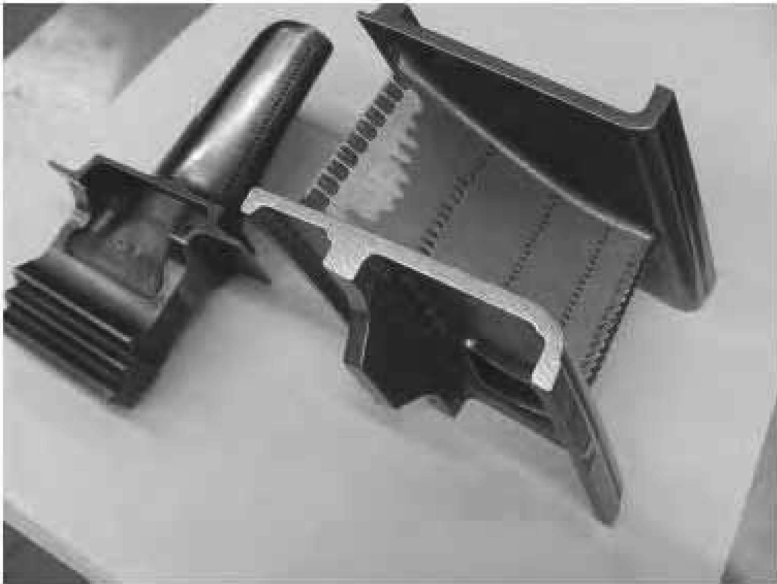
Figure 1: Turbine blade built from super-alloy with vanes for cooling, reproduced from Shillig [10]
