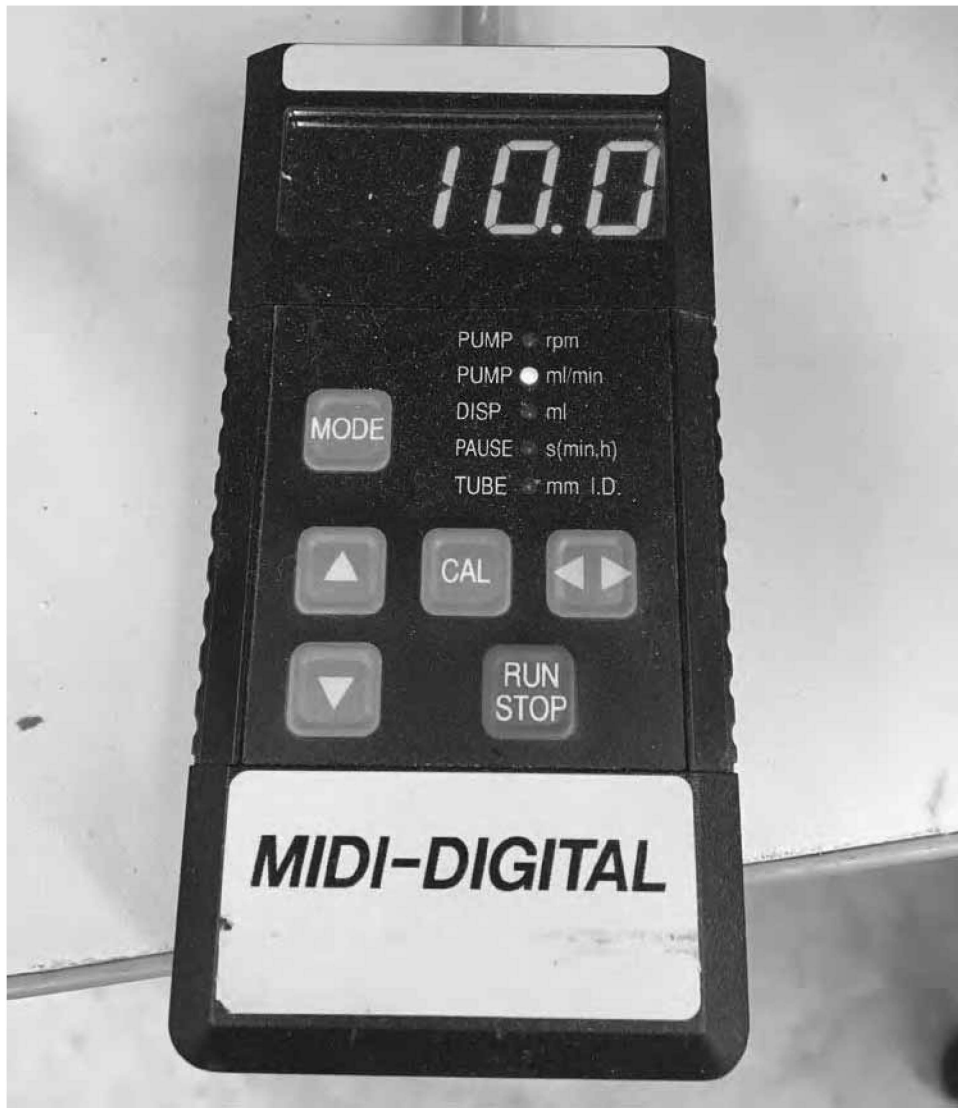
Figure 49. Flow rate controller. The red “RUN STOP” button is used to stop and start the flow of distilled water. Flow rate is adjusted using the vertical blue arrow buttons
