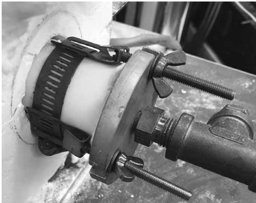
Figure 45. Nose of steam generator (right) secured to alumina tube which is inserted into preheaters (left).
