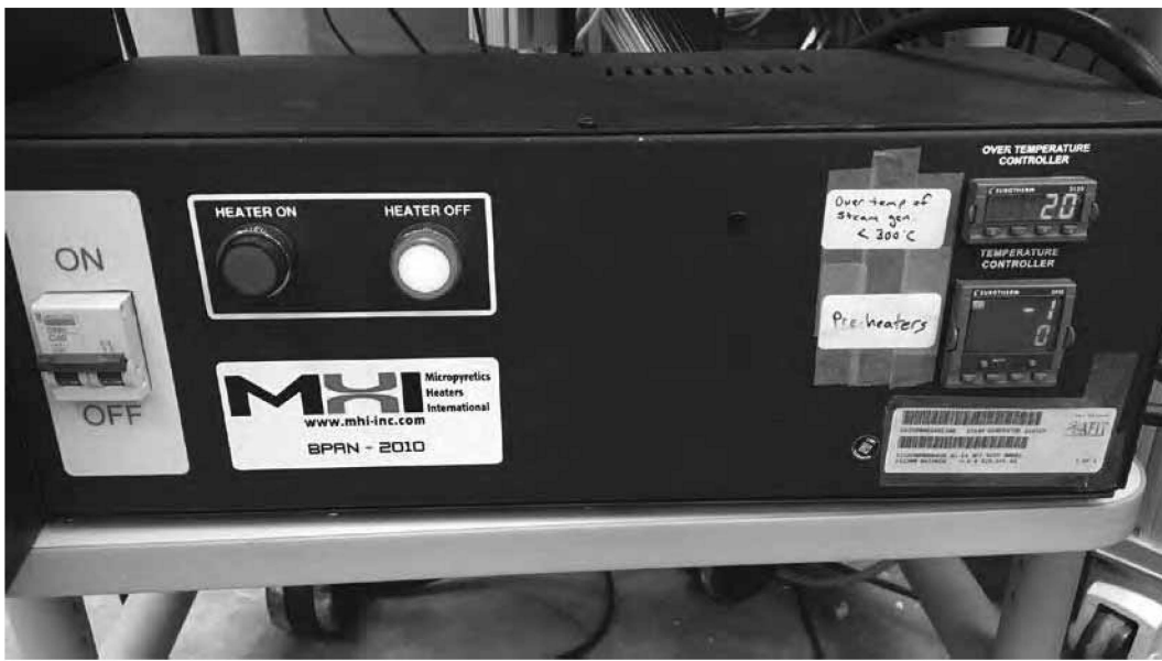
Figure 47. MHI BPAN-2010 control box. The switch on the left must be in the ON position and the HEATER ON light must be on in order for current to flow to the preheaters. As pictured, the switch is ON and the HEATER OFF light is on.
