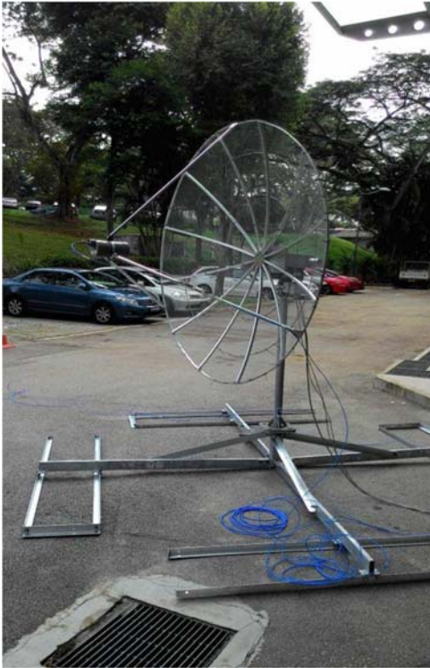
Figure 5-5 Completed mesh antenna with rotor and base structure
