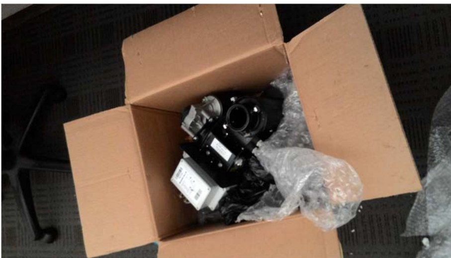
Figure 5-6 Rotor used to rotate the mesh antenna in both azimuthal and elevation direction
