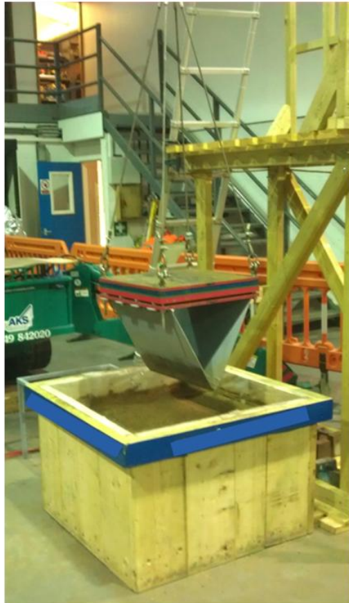
Figure 2. Wedge drop test for simulating wave impact pulse 3
