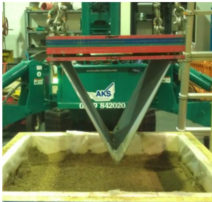
Figure C1. Test Platform including Wedge End View C1
