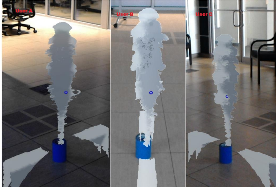
Fig. 3 Views from three Microsoft HoloLens devices showing the placement of a 3-D holographic object on top of a blue cylinder in the actual environment. From left to right, User A, User B, and User C as viewed from their positions as shown in Fig. 2.
