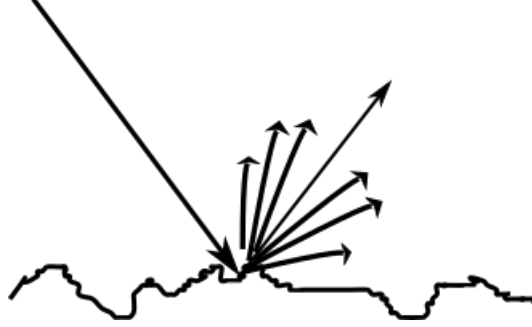
Figure 2.1. Light incident on a non-ideal surface.
