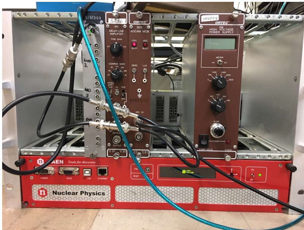
Figure 11. Components utilized in the experimental data acquisition. The settings for the voltage source, delay line amplifier, and multichannel analyzer are shown.
