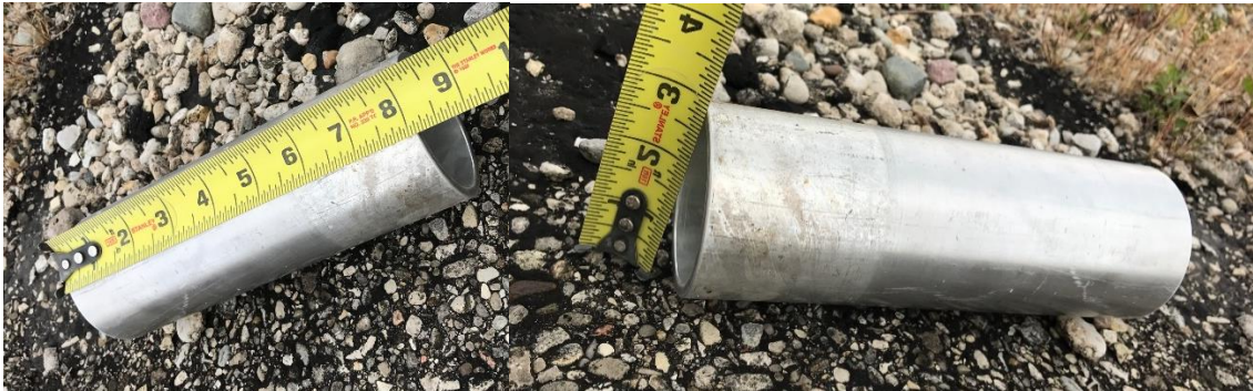
Figure 36: 3” by 8” pipe section length and diameter measured with tape measure
