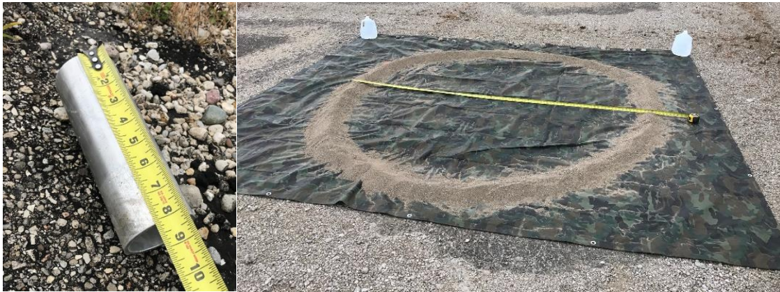
Figure 10: 3"x8" pipe section left, 96" dirt ring right
