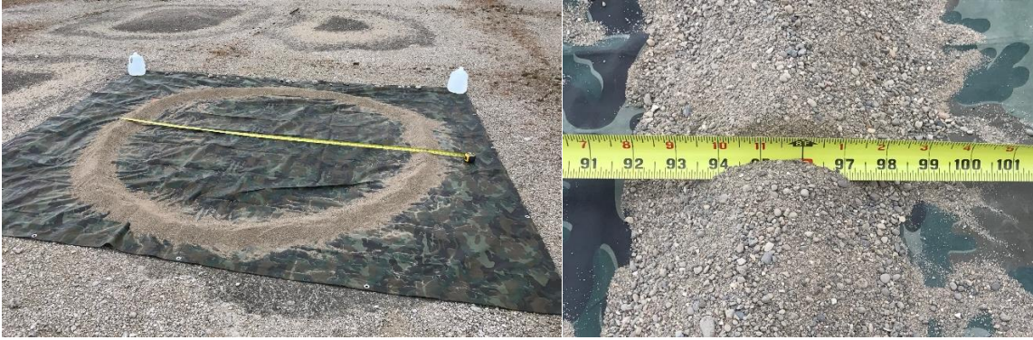
Figure 30: Test Ring Measured Diameter Approximately 96” with Tape Measure
