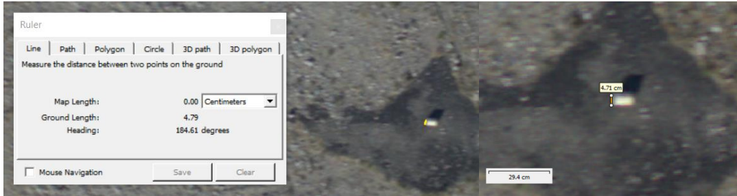
Figure 32: Flight 3B Measured Diameter of 2” x 3” Test Article GE left, Photoscan right
