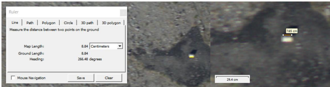
Figure 31: Flight 3B Measured Length of 2” x 3” Test Article GE left, Photoscan right
