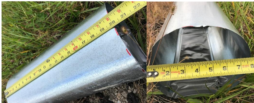
Figure 39: 8" by 20" Pipe Section Length and Diameter Measured with Tape Measure
