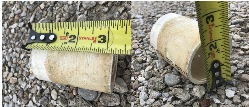
Figure 33: 2” by 3” Pipe Section Length and Diameter Measured with Tape Measure
