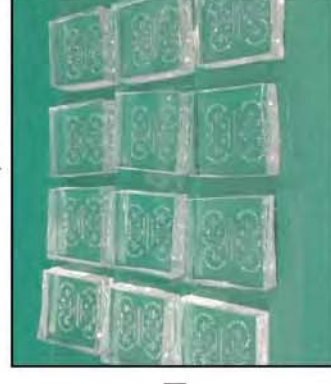
v. Cut PDMS into individual device "chips"
