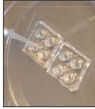
viii. Functionalize with ECM coating and seed cells
