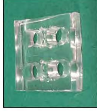
vi. Cut out seeding ports and media reservoirs
