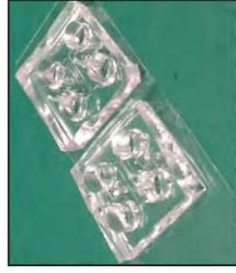
vii. Plasma treat and bind devices to cover glass
