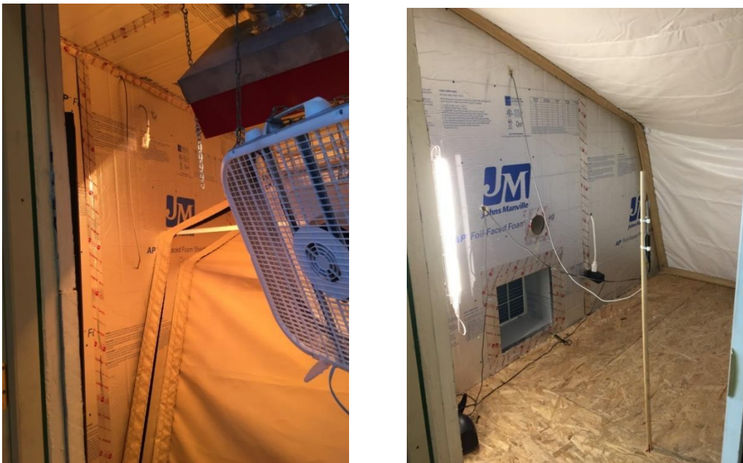
Figure 13: Hot box, climatic chamber (left) and metering chamber (right)
