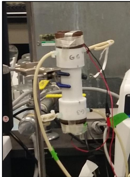
Figure 2: Dual Inlet/Outlet Reactor
