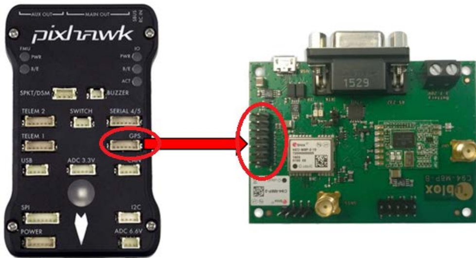
Figure 49. 3DR Pixhawk Flight Controller Integration to Ublox C94-M8P – GPS
