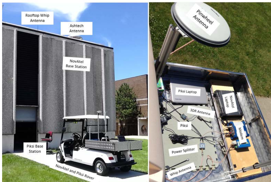
Figure 10. AFIT RTK System Shown in Parallel with Piksi RTK System via AFIT’s Mobile GPS Unit (Golf Cart)
