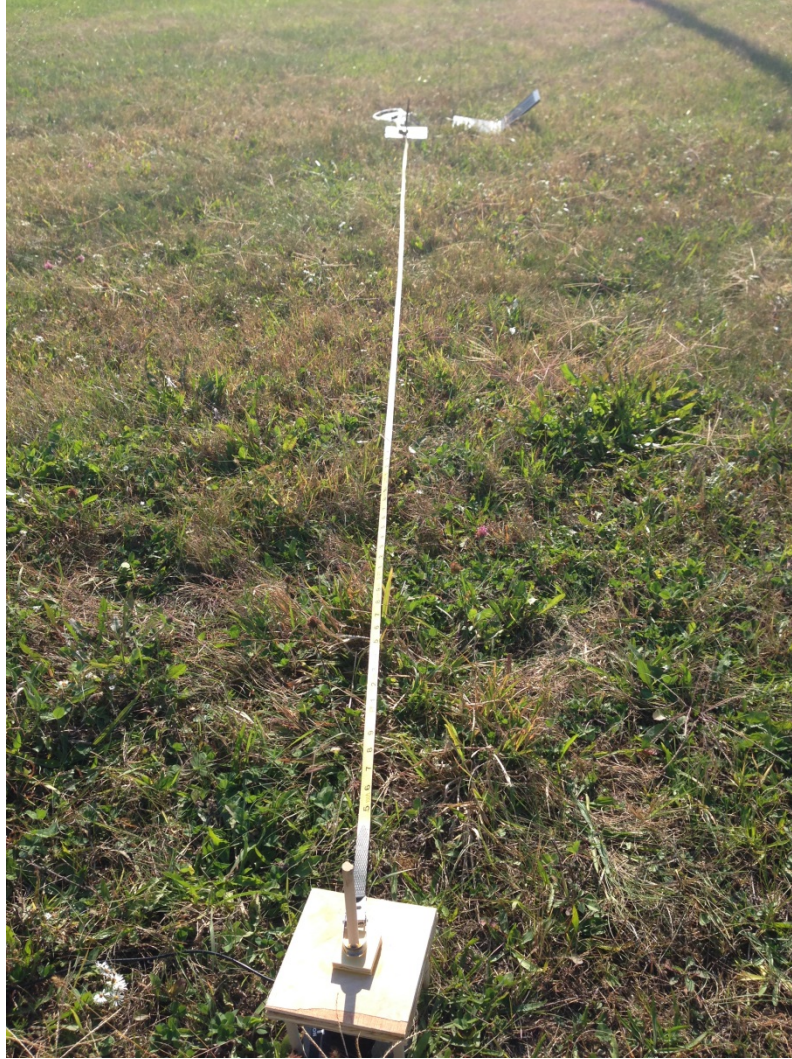
Figure 11. Relative Accuracy and Precision Test Setup (test # 5 and #6) – Known Distance of 15 Feet (4.572 m)
