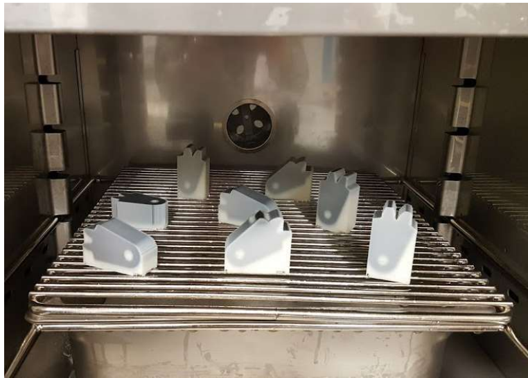
Figure 12: ProJet 3500 Parts during Post-Processing
