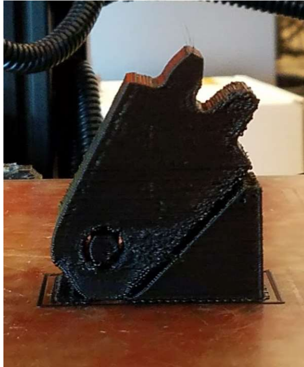
Figure 13: Lulzbot Print with Support Material
