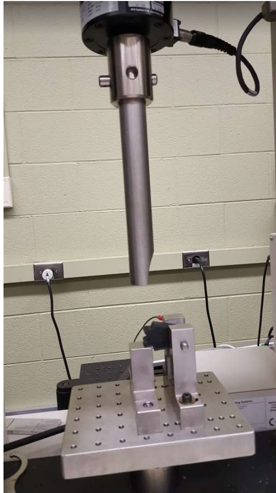
Figure 8: Final Gear Bending Test Fixture
