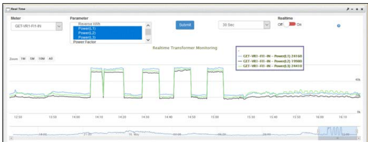
Figure 15. Power Monitoring Mode Output for 100 KVA High Variation Load Testing May 16, 2017
