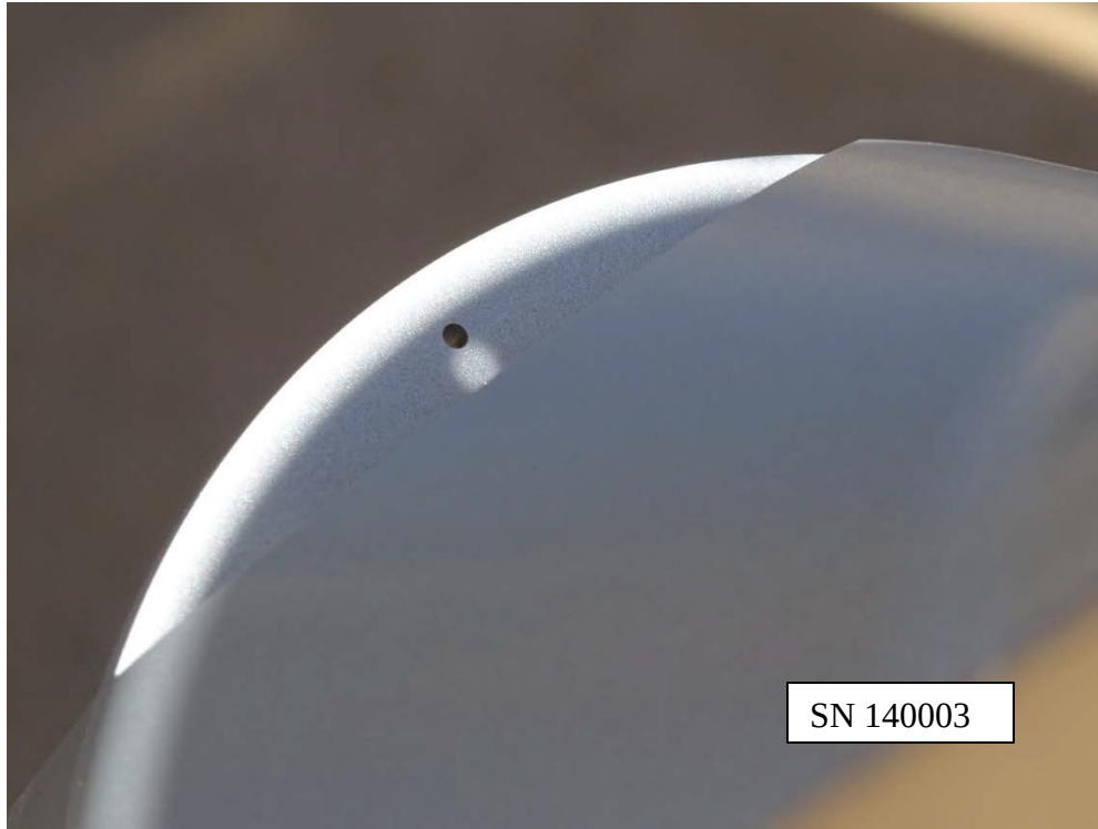
Figure 16. The alignment sunspot for DNI sensor (SN 140003), the cleaner of the two sensors in Figure 15. This misalignment is outside the Kipp and Zonen alignment specifications which can result in a false low reading for DNI. Note that the modules on this tracker indicated that the array was accurately aligned with the sun while the DNI sensor was misaligned with the sun. SN 140029 was within alignment specifications.
