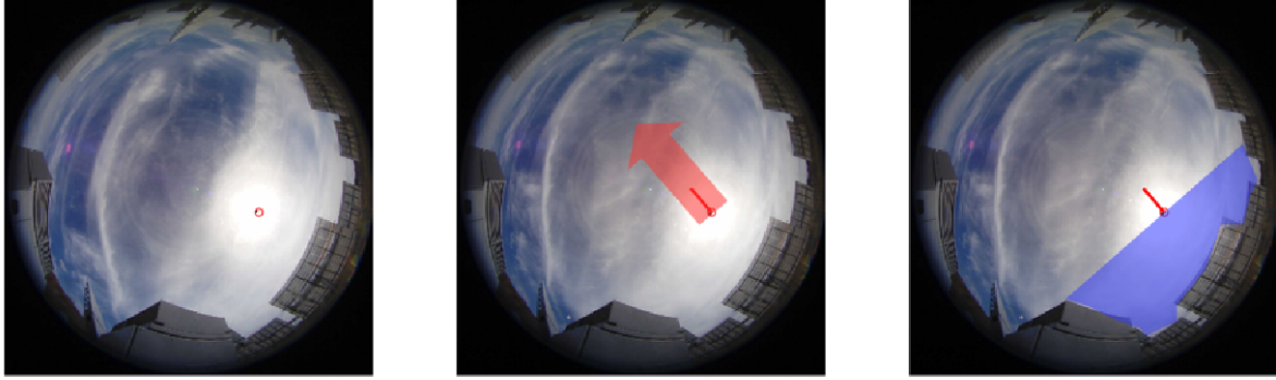
Figure 9: Example of how cloud motion detection is implemented in this work. By using two consecutive images (image at t_{issue} - 1 minute in the left panel and image at t_{issue} in the center panel) we can determine the cloud direction (red arrow in the center panel). Using this information we compute the image features for the portion of the sky that will influence DNI and PO in the next minutes (area highlighted in blue in the right panel).
