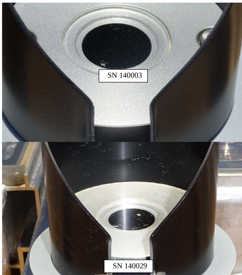
Fig. 2. (From site inspection) Both DNI sensors show soiling that will impact the resource measurements and performance evaluation for the plant. In the picture of SN 140003 it is difficult to see but minor soiling is noted. SN 140029 has readily visible soiling in the photograph that is estimated to be in the 1-3% loss range.
