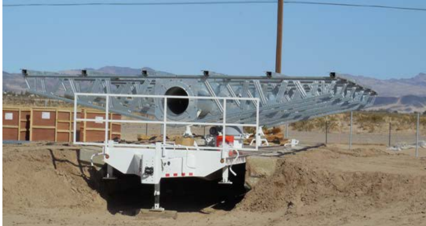
Figure 8. USTA Field Setup with Tracker Structure Mounted on Specialized Trailer
