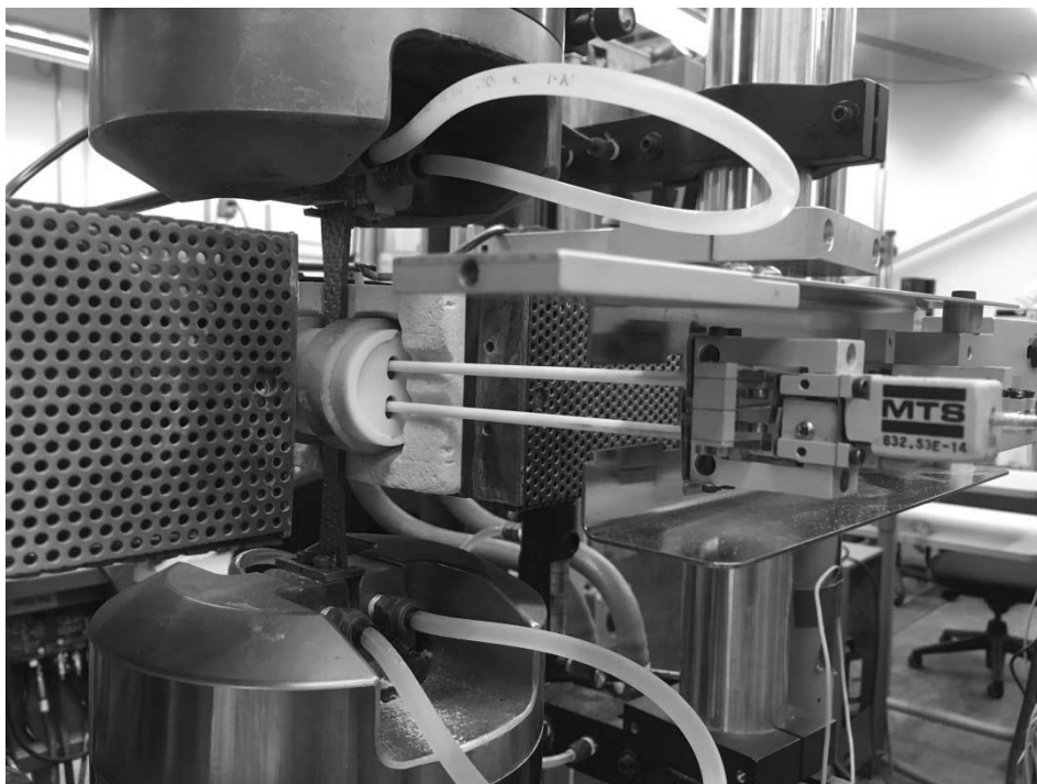
Figure 15: Furnace, susceptor and extensometer in preparation for testing.
