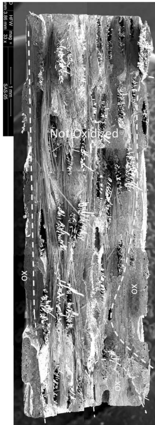
Figure A46: SEM micrograph of the fracture surface of specimen tested in fatigue at 1200°C in steam. \sigma_{\max} = 130 \text{ MPa} , N_f=3,201 .
