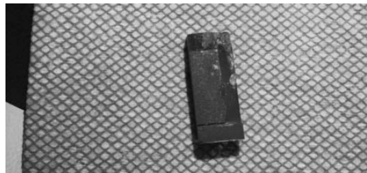
Figure A-195. Picture of HfB 2 -10SiC specimen that failed upon load up to 100 MPa at 1500°C.
