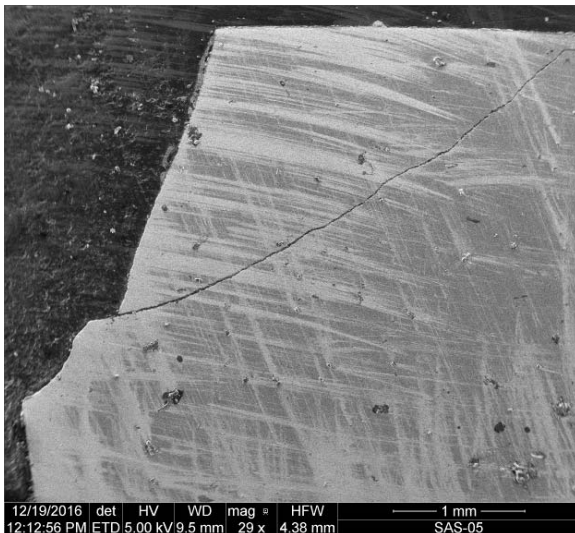
Figure A-58. Cross-sectional SEM micrograph of the \text{HfB}_2 -10% SiC specimen subjected to 1 h of compression creep at 8 MPa at 1500°C in air (failed upon load-up to 100MPa).
