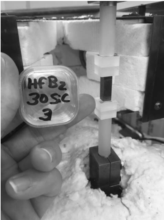
Figure A-197. Specimen loaded for compression creep testing.
