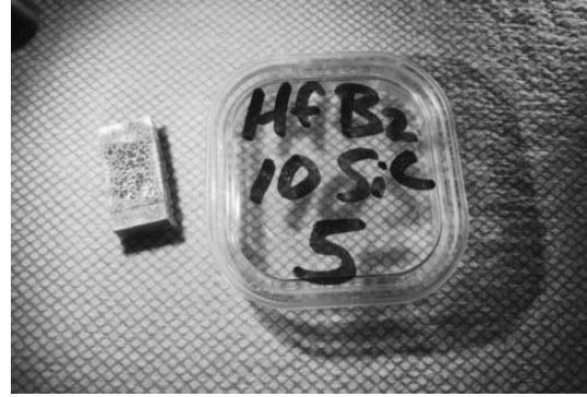
Figure A-186. Picture of \text{HfB}_2 -10SiC specimen subjected to 75 MPa compressive creep stress for 66.3 h at 1500°C.
