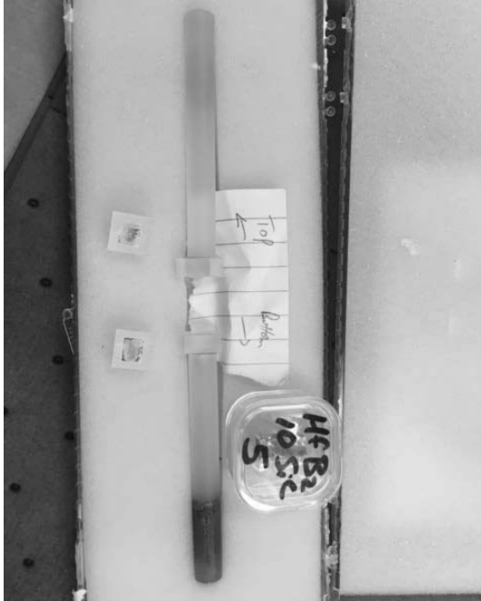
Figure A-208. Load train subjected compression creep of HfB 2 -10% SiC specimen at 75 MPa for 66.3 h with 4 random orientation spacers.
