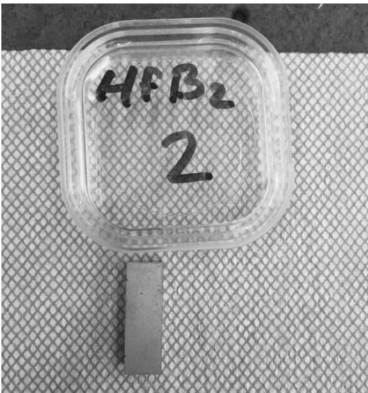
Figure A-213. Picture of a HfB 2 specimen prior to being subjected to compression creep at 75 MPa for 20h at 1500°C in air.
