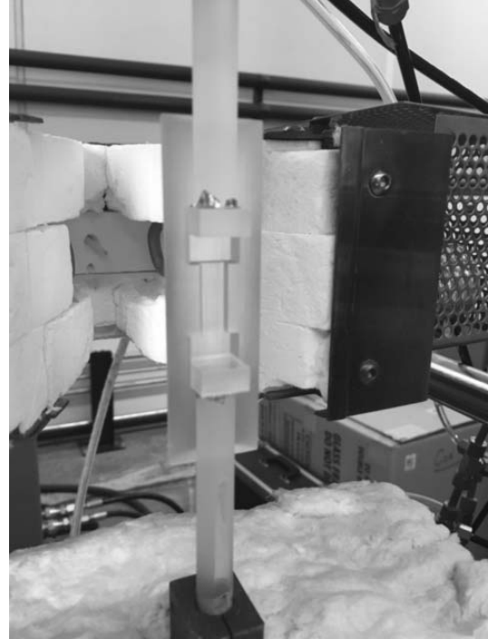
Figure A-229. Initial testing of alignment tool during temperature calibrations.
