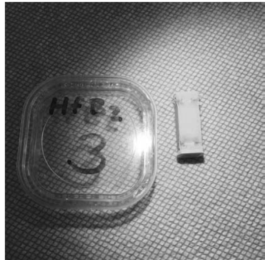
Figure A-179. Picture of \text{HfB}_2 specimen subjected to 75 MPa compressive creep stress for 30 h at 1500°C.
