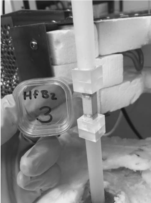
Figure A-216. Picture of load train with a HfB 2 specimen after being subjected to compression creep at 75 MPa for 30h at 1500°C in air.
