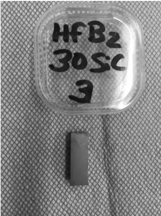
Figure A-201. Pre-test images of a HfB 2 -30% to be subjected to compression creep at 100 MPa for 8.8 h.
