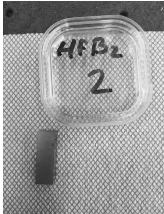
Figure A-211. Picture of a HfB 2 specimen prior to being subjected to compression creep at 75 MPa for 20h at 1500°C in air.
