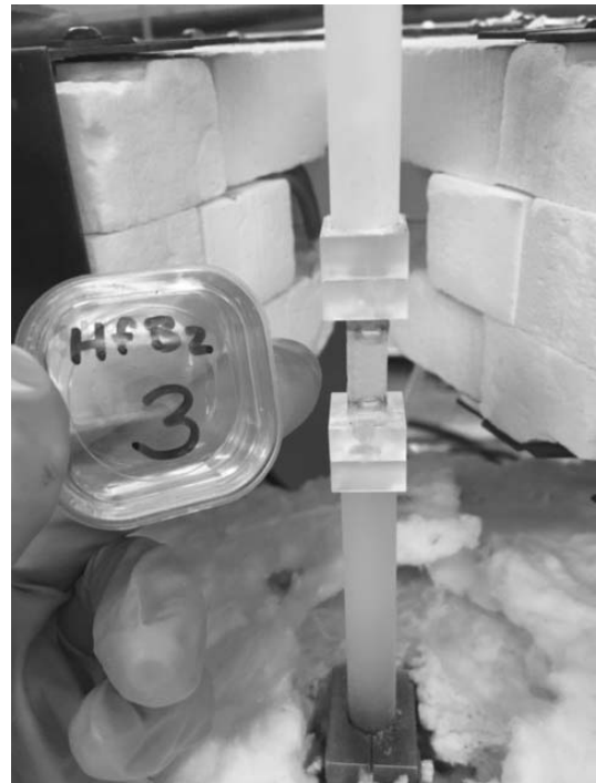
Figure A-215. Picture of load train with a HfB 2 specimen after being subjected to compression creep at 75 MPa for 30h at 1500°C in air.
