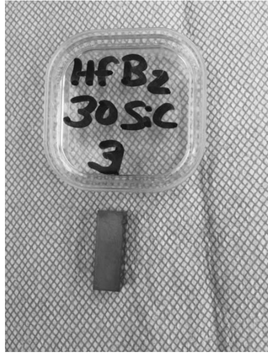
Figure A-202. Pre-test images of a HfB 2 -30% to be subjected to compression creep at 100 MPa for 8.8 h.
