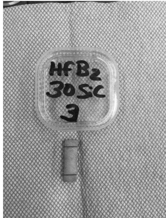
Figure A-203. Pre-test images of a HfB 2 -30% to be subjected to compression creep at 100 MPa for 8.8 h.
