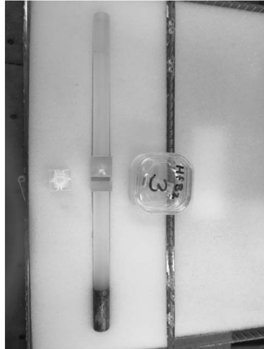
Figure A-207. Load train subjected compression creep of \text{HfB}_2 specimen at 75 MPa for 30 h with four random orientation spacers.
