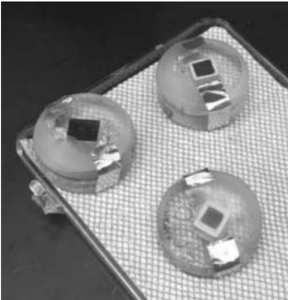
Figure A-169. Picture of post-test specimens prepared for SEM imagery.
