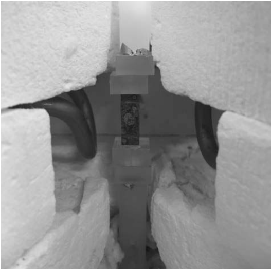
Figure A-228. Load train of HfB 2 -10% SiC specimen after a compression creep test at 75 MPa for 66.3 h at 1500°C in air.
