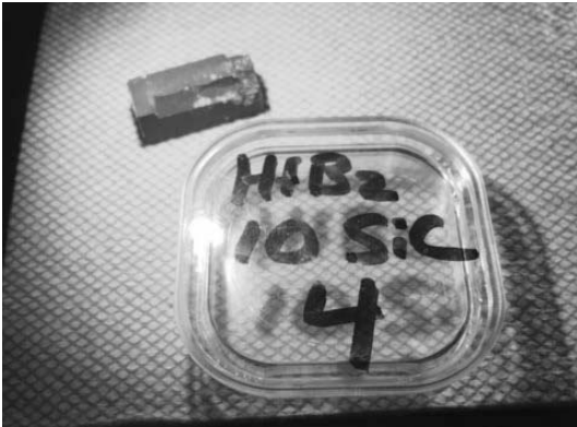
Figure A-190. Picture of HfB 2 -10SiC specimen that failed upon load up to 100 MPa at 1500°C.
