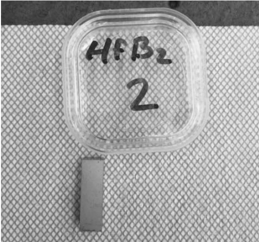
Figure A-212. Picture of a HfB 2 specimen prior to being subjected to compression creep at 75 MPa for 20h at 1500°C in air.
