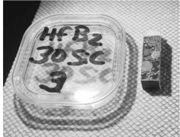
Figure A-170. Picture of \text{HfB}_2 -30% SiC specimen subjected to 100 MPa compressive creep stress for 8.8 h at 1500°C.
