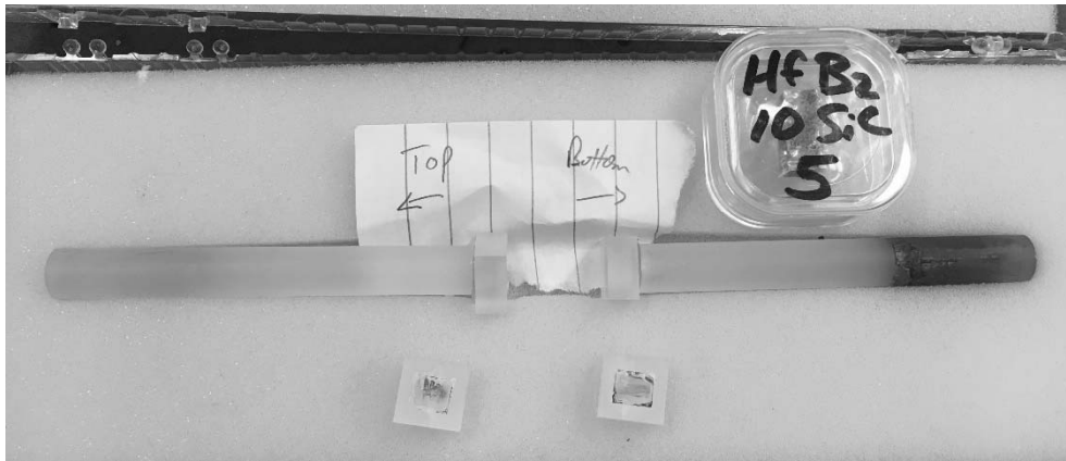
Figure 19. YAG Rods and Sapphire Spacers used in the 75 MPa compression creep test of 66-h duration. Note depressions in the sapphire spacers indicative of substantial superplastic deformation.
