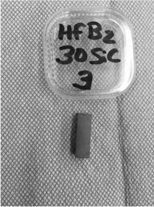
Figure A-200. Pre-test images of a HfB 2 -30% to be subjected to compression creep at 100 MPa for 8.8 h.
