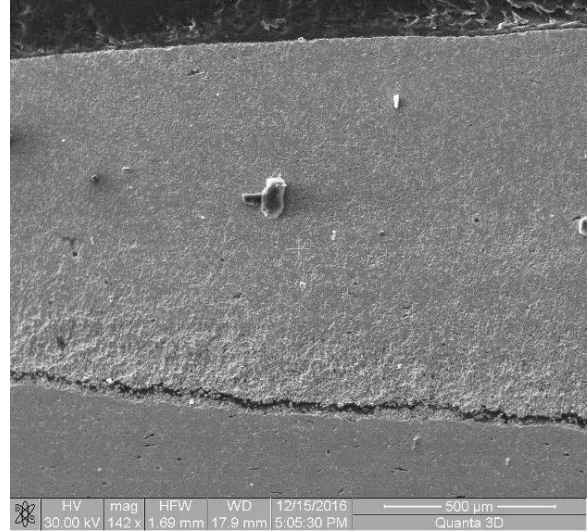
Figure A-39. Cross-sectional SEM micrograph of the HfB 2 specimen subjected to 30 h of compression creep at 75 MPa at 1500°C in air.
