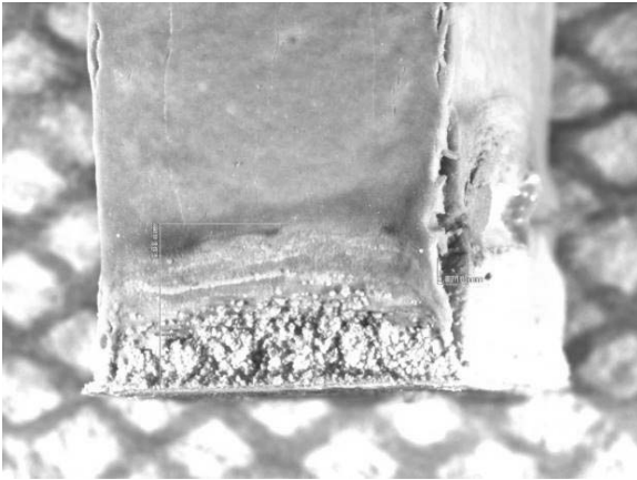
Figure A-154. Optical micrograph of the \text{HfB}_2 specimen subjected to 30 h of compression creep at 75 MPa at 1500^\circ\text{C} .
