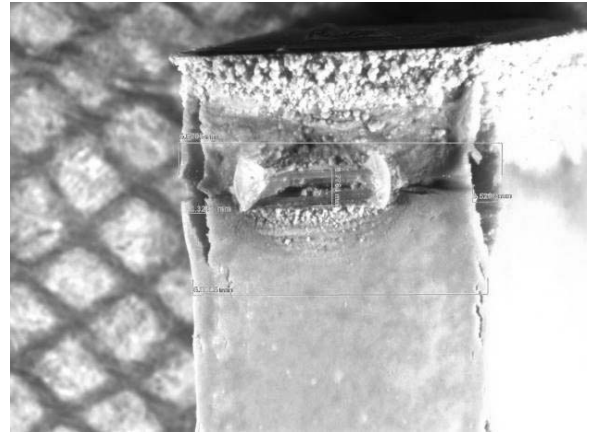
Figure A-152. Optical micrograph of the HfB 2 specimen subjected to 30 h of compression creep at 75 MPa at 1500°C. Note the scale buildup and discoloration near ends. Depression at extensometer groove includes two broken pieces of sapphire extensometer rod.
