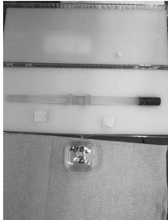
Figure A-199. Load train after testing HfB 2 specimen for 20 h at 75 MPa in air at 1500°C with four random orientation spacers.
