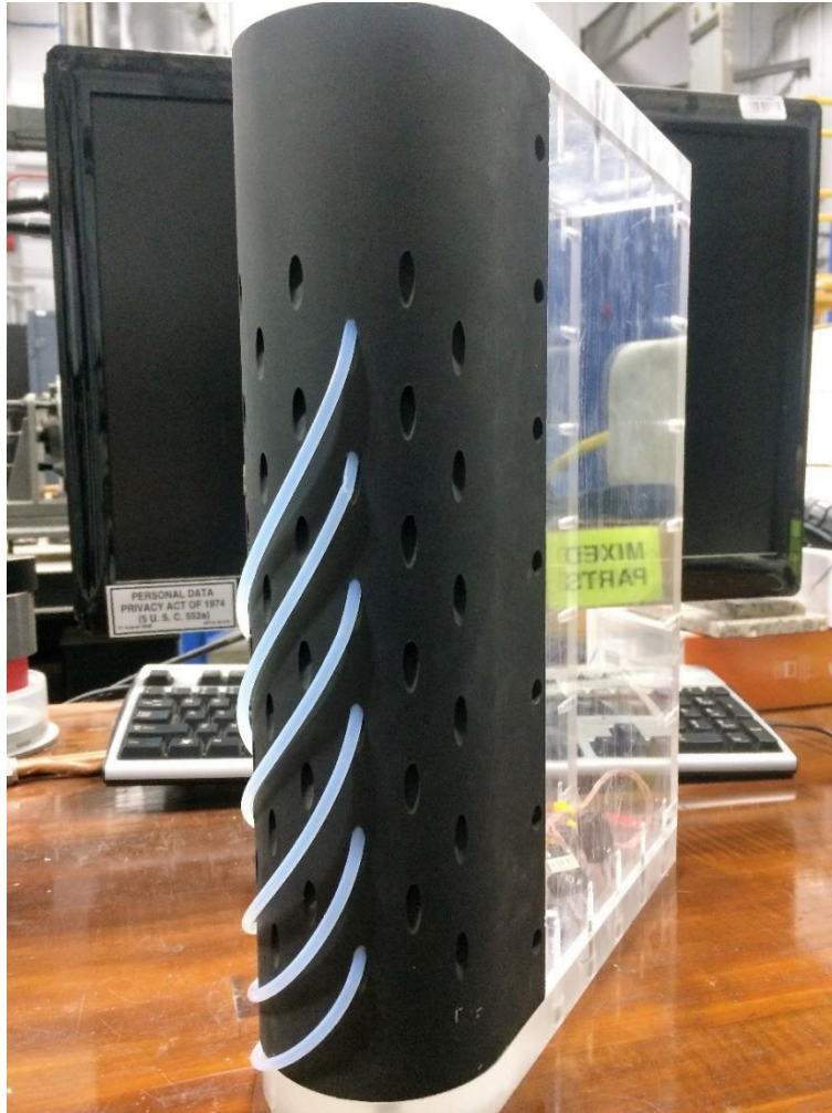
Figure 49: Experimental model with tubes installed to remove film cooling
