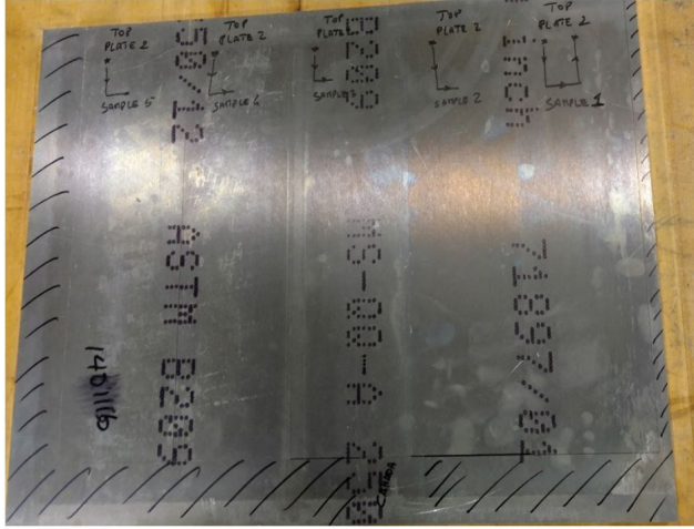
Figure 3.1. Material size as delivered, five specimens machined out of each plate. Hashed lines in figure show unused material.
