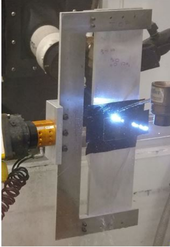
Figure 3.14. Circle Spot Laser Peening Fixture
