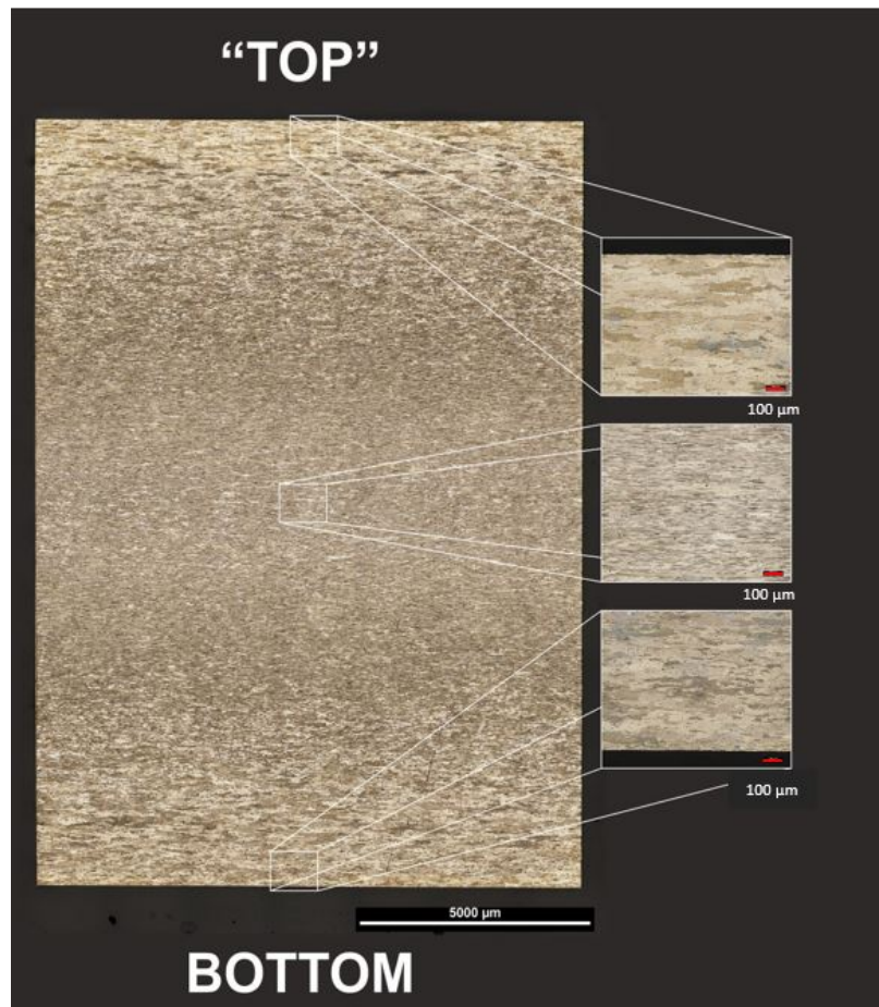
Figure 3.7. Grain structure through the thickness of as received material. Note variations in grain sizes from top/bottom edges to the center.
