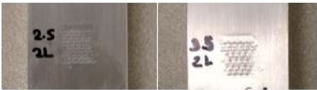
Figure 3.11. Energy Level Test Samples. (Left image shows the test with a laser energy of 2.5 J with two applications. Right show the test with a laser energy of 3.5 J with two applications.)
