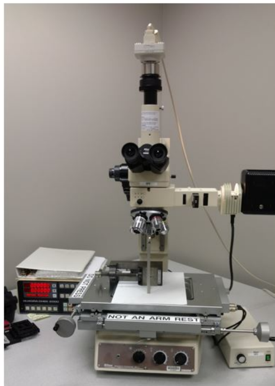
Figure 3.28. Optical microscope with integrated XY measuring table.
