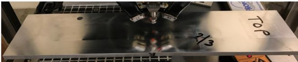
Figure 3.27. Peened Residual Stress Measurement Area for X-Ray Diffraction
