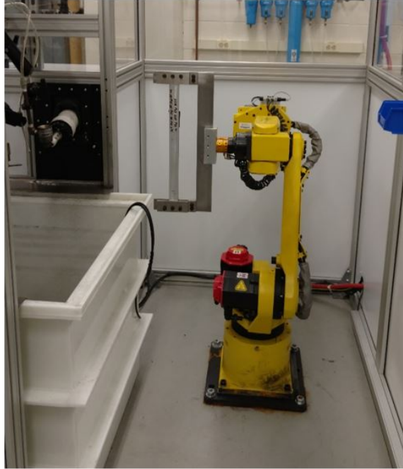
Figure 3.17. Robotic Arm Used to Relocate Sample in Beam's Path
