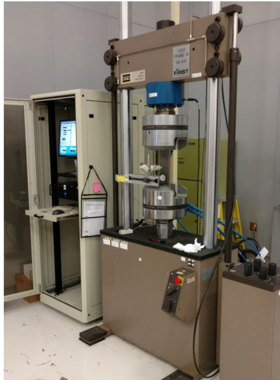
Figure 3.6. MTS Load cell with traveling microscope attached
