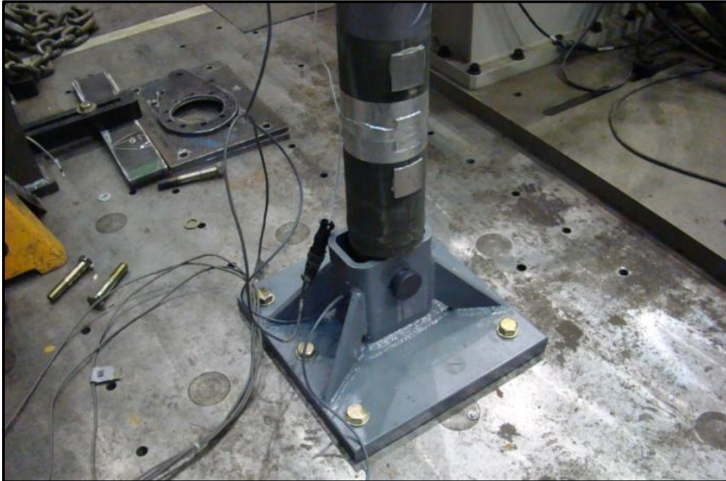
Figure 8. Tow bar calibration fixture fastened to a bedplate.
