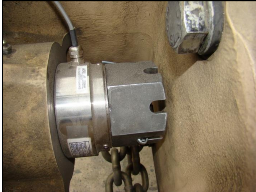
Figure 2. Modified pintle mount assembly with custom load cell installed.
