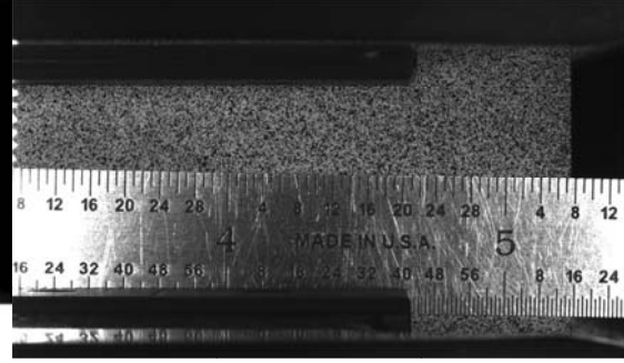
Figure 3.15. DIC Spatial Calibration
