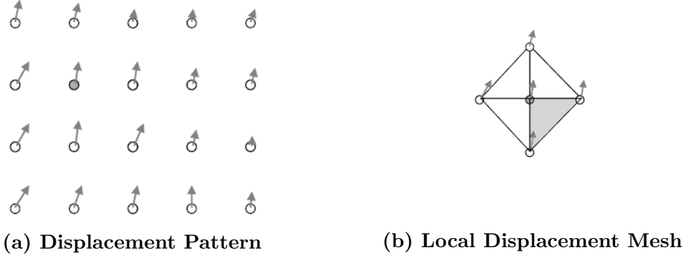
Figure 2.21. DIC Displacement Vectors [27]
