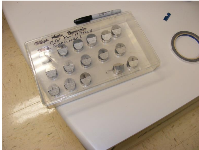
Figure 30. Hi-Nicalon TM S fiber tow specimens tested in creep at 900°C in air and in silicic acid-saturated steam prepared for examination with an SEM
